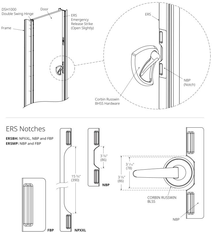
The ERS notches are designed to clear a variety of door hardware trim with a 2<sup>3</sup>/<sub>4</sub>" backset. For example the NBP notch is large enough to clear most cyclindrical locking levers with rose trim, including the Corbin Russwin Behavioral Health Series Lever (BLSS).
