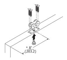
\*From door edge to centerline of hanger bolt and plate.
