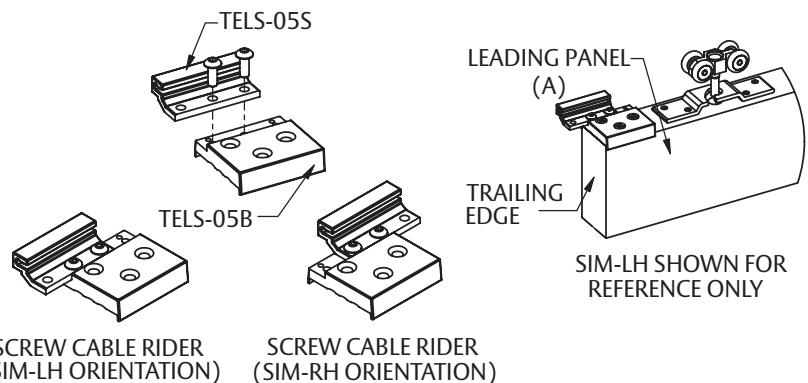
Use 1-1/2" wood screws (PBS12150SP10BLR) to secure Screw Cable Rider Assembly to top of Panel A.
