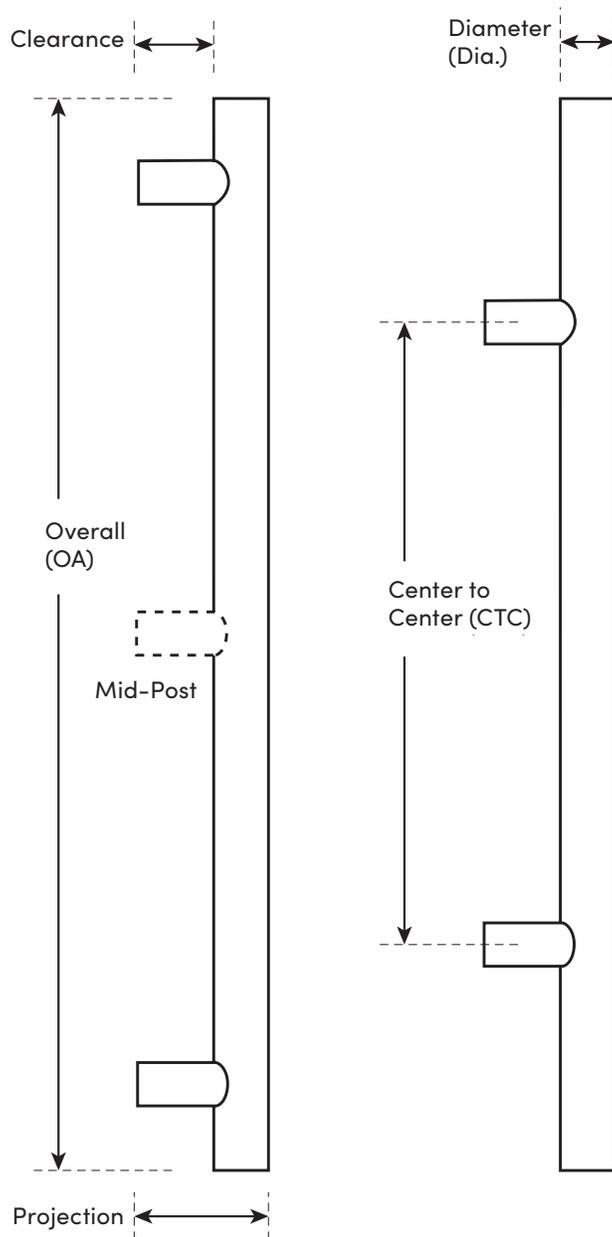
On long pulls, post can be positioned closer to each other and farther away from ends as a strategy to avoid mid-post if door condition permits.
