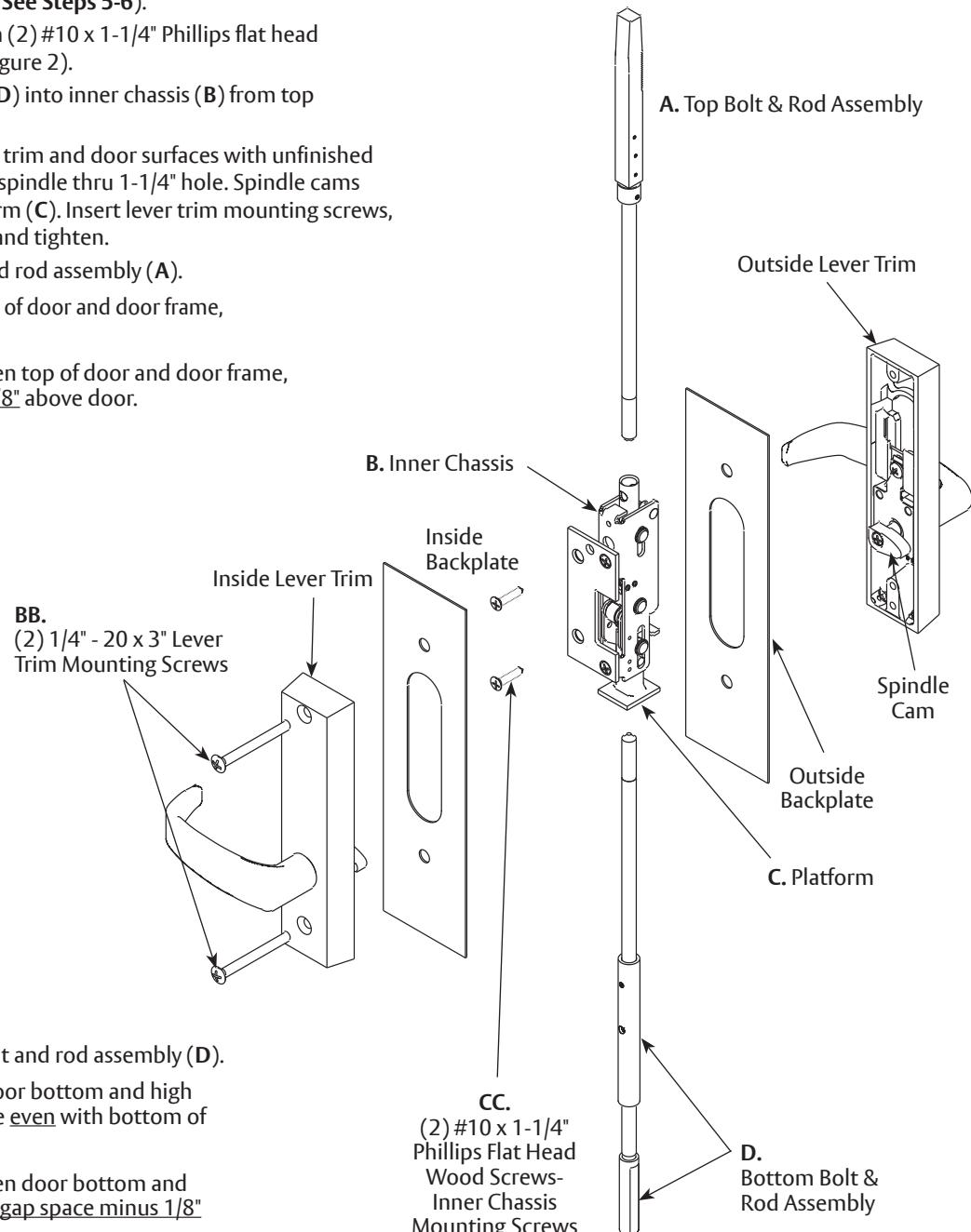
6. Use inside trim to adjust bottom bolt and rod assembly (D).
