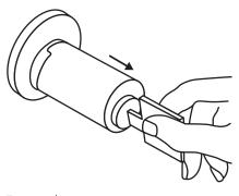
To remove key return key to vertical position position and withdraw.
