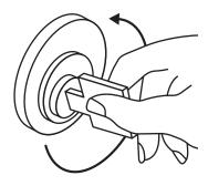
With key in this position pull out cylinder.
