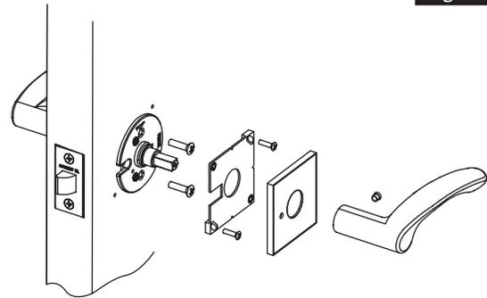
Note: To level plate, place a right angle square on the flat portion of the mounting plate.
