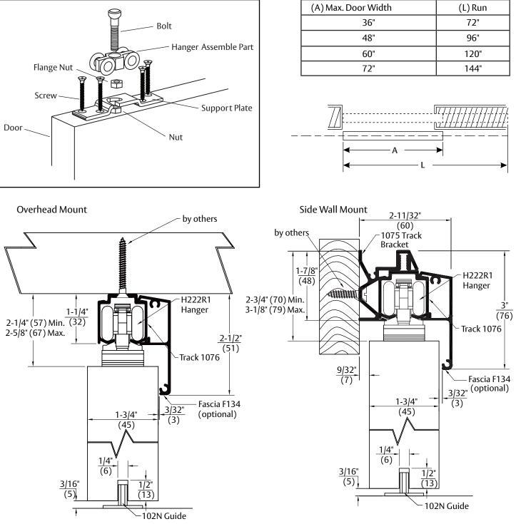
\* When using fascia, offset hanger foot 1/8" (3) closer to fascia face of the door.
