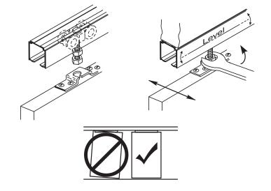
7. Install and secure retaining stops.
