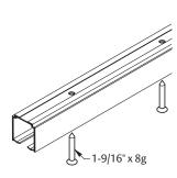
Note: Place fasteners at each end and no more than 24" (610) in between.
