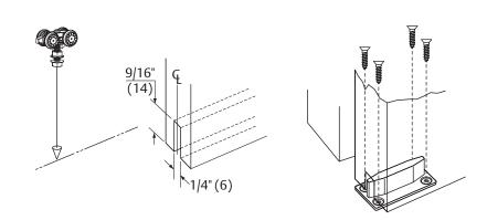
6. Attach door panel and adjust until level.
