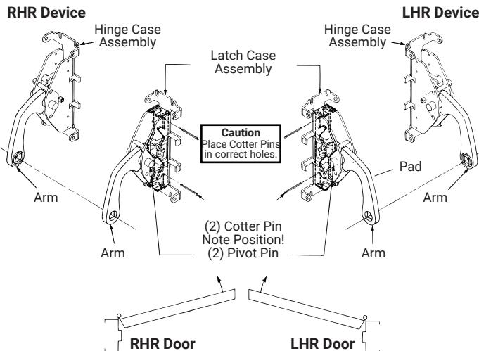
**Notes:** Complete device required to change hands, arms are swapped between latch and hinge cases, only essential components shown or highlighted, for clarity.
