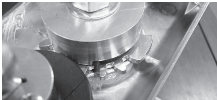
Spring orientation for right hand reverse operation
