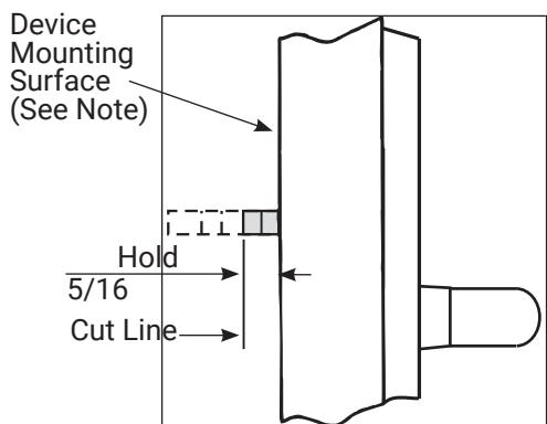
**Note:** Measure from device seat. (Door face as shown)
