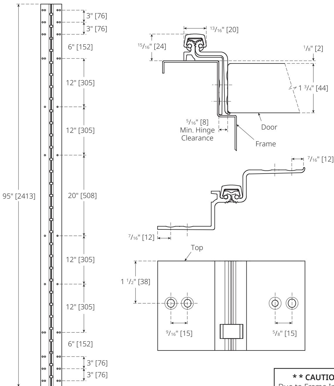
Additional clearance needed for bevelled edge hinge side of door.
