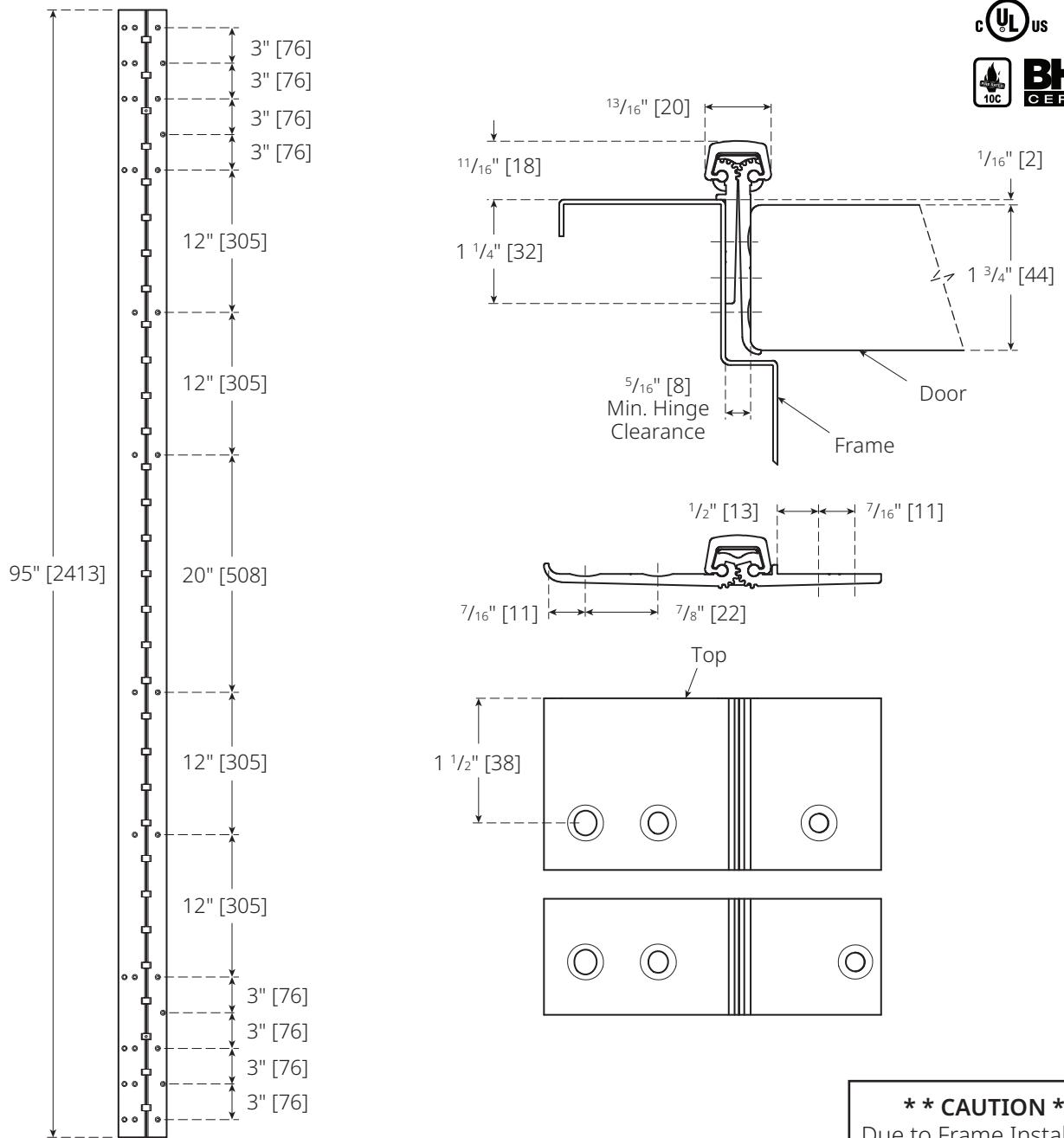
Additional clearance needed for bevelled edge hinge side of door.
