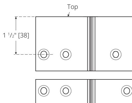
Additional clearance needed for bevelled edge hinge side of door.
