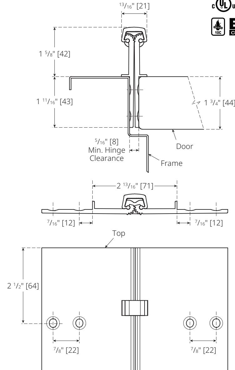
Additional clearance needed for bevelled edge hinge side of door.
