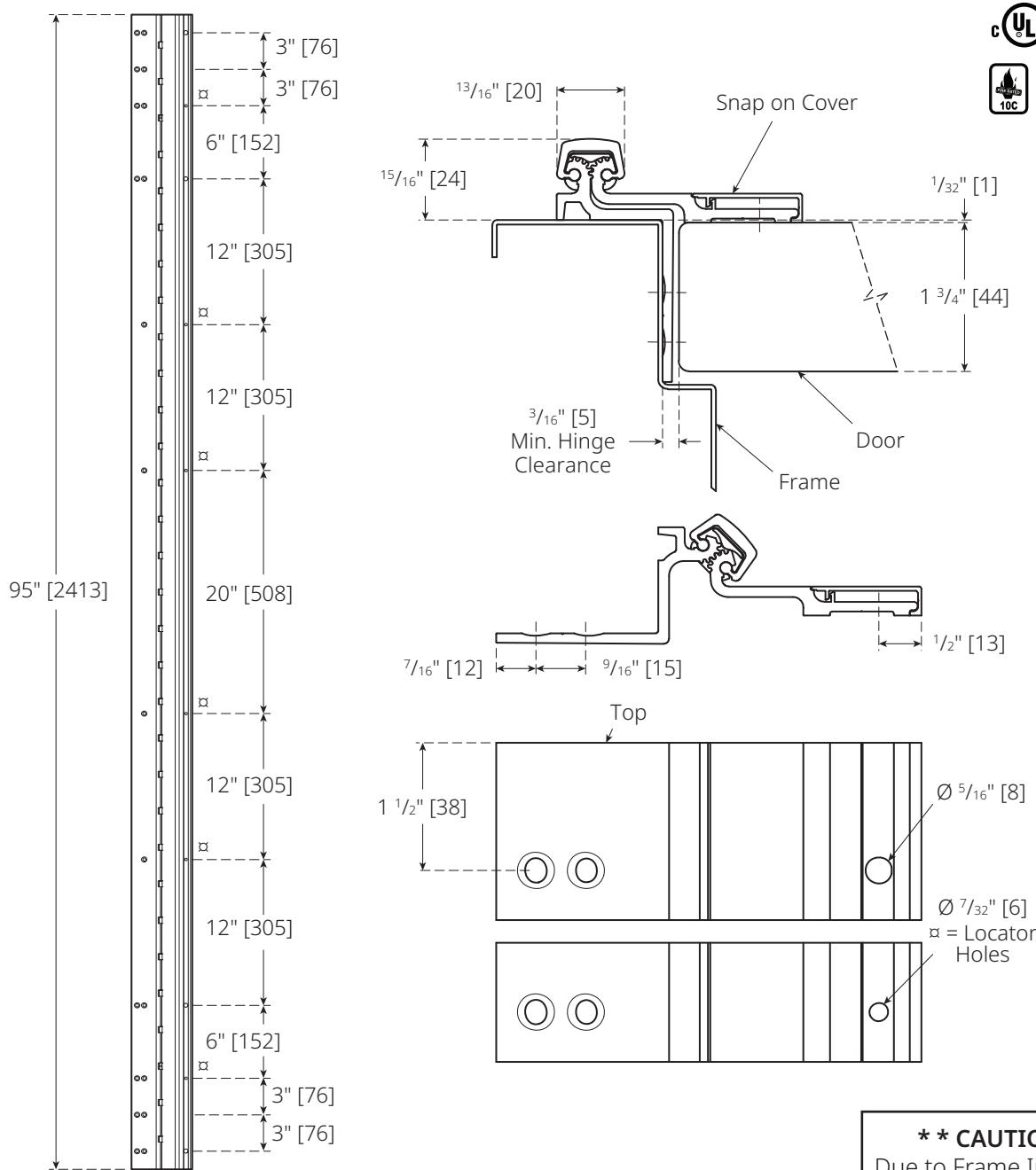
Additional clearance needed for bevelled edge hinge side of door.
