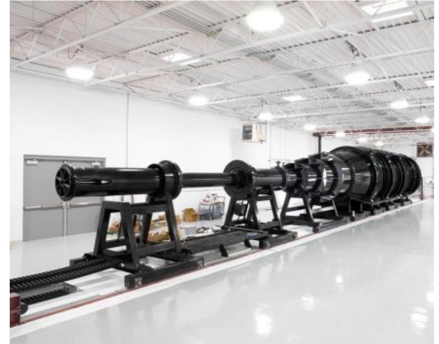
Shock Tube - ASTM F292712, Standard Test Method for Door Systems Subject to Air blast Loadings
