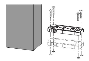
**3**. Use floor plate adjustments to align patch fitting in opening.
