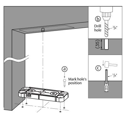
2. Install floor plate using four M8 x 30MM bolts.
