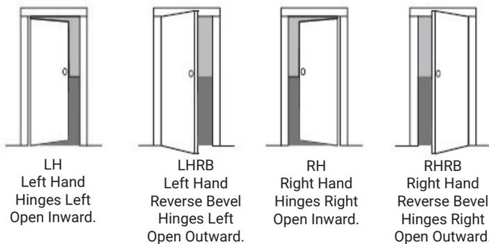
**NOTE:** Stand on outside of locked door when determining door hand.
