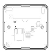
The "LINK" LED on the Ethernet connector indicates both status of the Ethernet Link level and if communication is ongoing.
