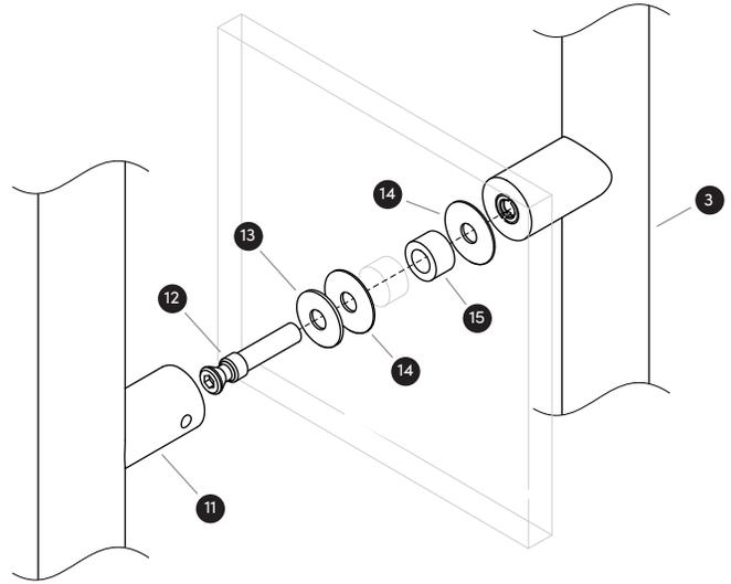
Alignment Bushing and Spacer available on Wood, Metal, and Storefront Doors - this replaces items 14 and 15 in the above image referencing a glass door.
