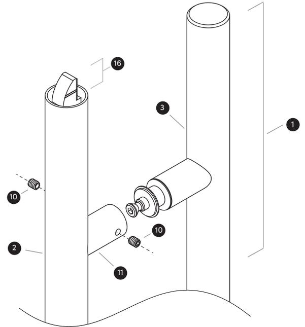
**NOTE:** When installing the full height bottom tubes or horizontal push bar on the thumbturn side, the thumbturn may have to be turned to the unlocked position in order to be able to slide the tube into place.
