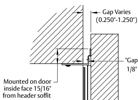
2. Remove backing from gasket and adhere to face of door at marked location; pressing firmly to ensure adequate bonding.
