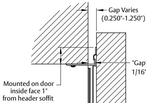
If using PY900 in alternate configuration, locate top of gasket on door 15/16" higher than head soffit.
