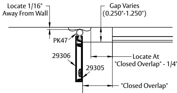
2. With door in the fully closed position, locate metal base (p/n 29305) on door edge so that bulb gasket is 1/16" to 3/32" away from the wall or frame.
