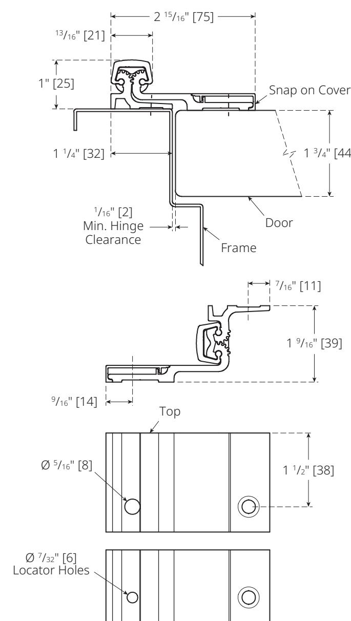
Additional clearance needed for bevelled edge hinge side of door.
