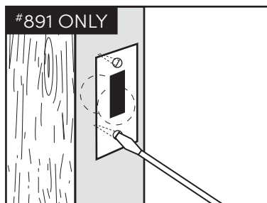
7. Screw strike plate into position using #6 x 5/8" flat head wood screws.
