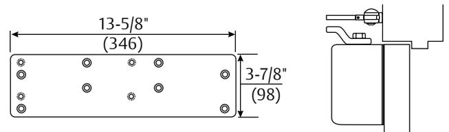
**Narrow Top Rail - 7786 Drop Plate:** For use where the narrow top rail of the door prevents the closer from being mounted directly to the door surface. This drop plate must be used for closer mounted on a top rail between 1-7/8" and 3-3/8" (48 and 86mm) in height.
