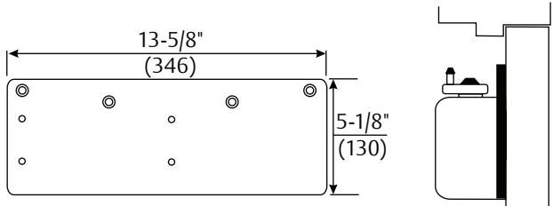
**Narrow Top Rail - 7788 Drop Plate:** For use where a narrow top rail prevents the closer from being mounted directly to the door surface. This drop plate can be used to mount a closer on a top rail as narrow as 2-3/8" (60mm) in height.
