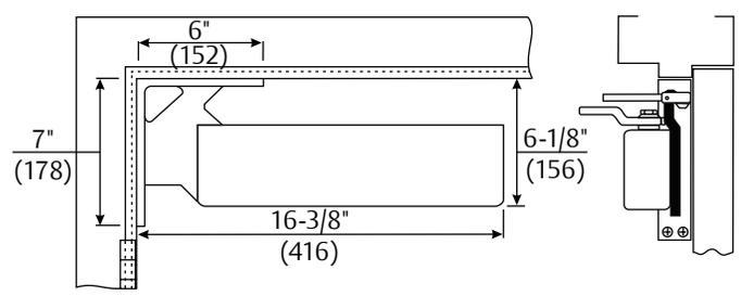
**Mounting Opposite Hinge Side - 7798 Standard Drop Corner Bracket:** For use where it is desired to mount a regular arm non-hold open closer.
