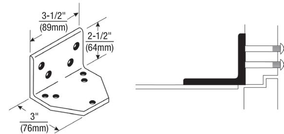
**Flush Rabbeted Transom - 2019L Angle Bracket:** For use where flush transom conditions prevent mounting of the standard soffit plate. This bracket is used in combination with the arm's soffit plate.
