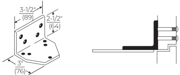
**Standard - 2019S Spacer Block:** For use where a narrow frame soffit does not provide adequate support for the soffit plate. Supplied standard with all Parallel Rigid arm closers.
