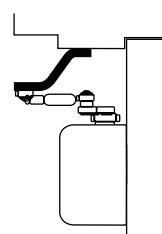
**Flush Transom - 2022 Angle Bracket:** For use where rabbeted or flush transom conditions prevent installation of a soffit plate. Used in combination with the 1618 soffit plate, or may be used in combination with the 2018S soffit plate when it is necessary for the closer arm to clear a separate overhead door holder.
