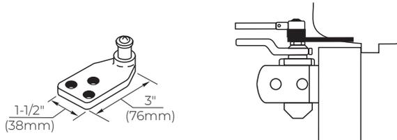
**Molded/Bull Nose Trim - 2403B Bracket:** For use where the door frame has molded or bull nose trim which will not accept a standard non-hold open shoe. The bracket is mortised into the frame rabbet, and projects beyond the face of the frame. It will accommodate a frame rabbet up to 2" (51mm) deep.
