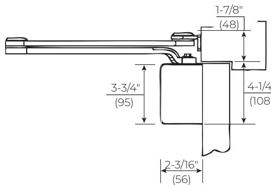
Mounting holes for closer body are spaced 2-3/8" (60mm) vertically x 6-3/4" (171mm) horizontally.
