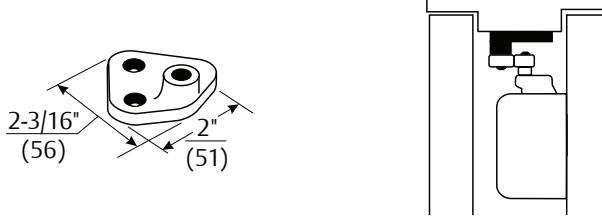
**Standard Installation - 1618 Soffit Plate:** Supplied standard with parallel arm closers. It can be mounted where the frame soffit is as narrow as 1" (25mm). Specify 1618A-SS for stainless steel soffit plate.
