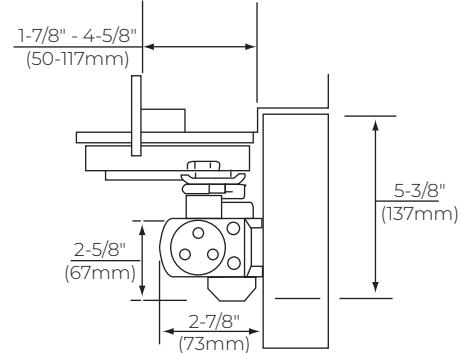
Mounting holes for closer body are spaced 3/4" (19mm) vertically x 9-1/16" (230mm) horizontally.
