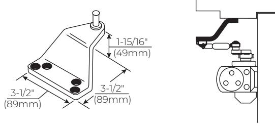
**Flush Transom - 2022 Angle Bracket:** For use where rabbeted or flush transom conditions prevent installation of a soffit plate. Used in combination with the 1618A soffit plate, or may be used in combination with the 2018S soffit plate when it is necessary for the closer arm to clear a separate overhead door holder.
