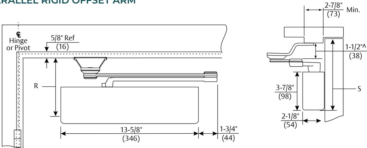
Mounting holes for closer body are spaced 2-3/8" (60mm) vertically x 6-3/4" (171mm) horizontally.
