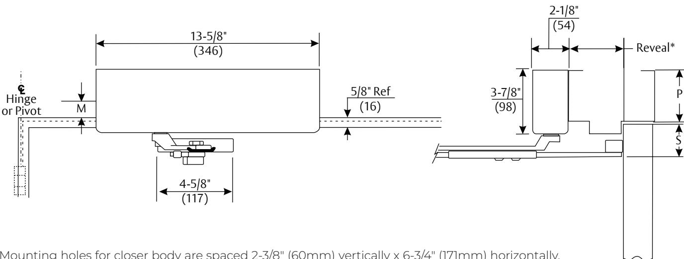
Mounting holes for closer body are spaced 2-3/8" (60mm) vertically x 6-3/4" (171mm) horizontally.
