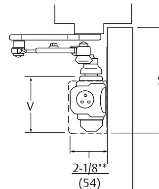
Mounting holes for closer body are spaced 3/4" (19mm) vertically x 12" (305mm) horizontally.
