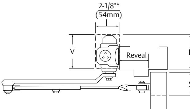
Mounting holes for closer body are spaced 3/4" (19mm) vertically x 12" (305mm) horizontally.
