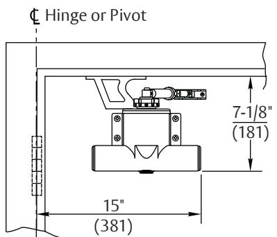
**Soffit Mounting - 1-B/F Soffit Bracket:**
