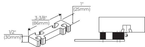
**Clearance/Support Blade Stop - 6891 Spacer Block:** For use where the door frame has a blade stop and the soffit plate must be mounted on the frame rabbet. This accessory is used in combination with the standard 2019S Spacer Block to provide clearance of the blade stop. For clearance of 5/8" (16mm) high-frame stop.
