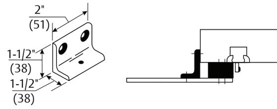
**Flush Rabbeted Transom - 2019L Angle Bracket:** For use where flush transom conditions prevent mounting of the standard soffit plate. This bracket is used in combination with the standard soffit plate.
