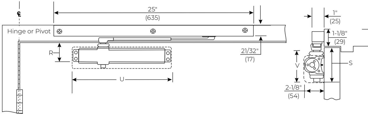
Mounting holes for closer body are spaced  $3/4"$  (19mm) vertically x  $12"$  (305mm) horizontally.
