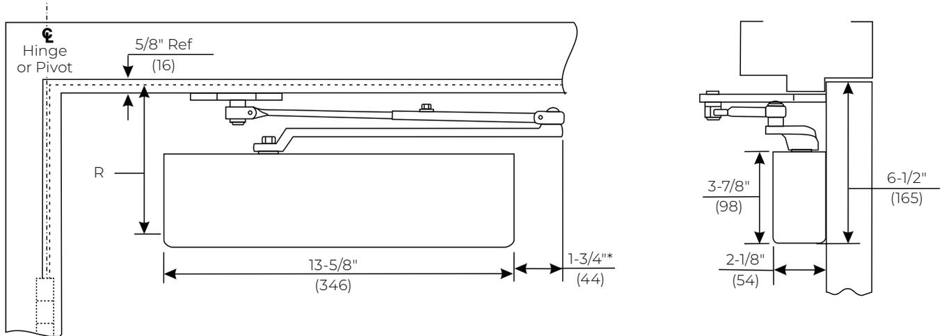
Mounting holes for closer body are spaced 2-3/8" (86mm) vertically x 6-3/4" (171mm) horizontally.
