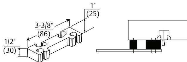
**Narrow Frame - 6890 Support Bracket:** For use where the frame is narrow, and the soffit plate cannot be mounted directly to the frame soffit or rabbet. Used in combination with the 6891 Spacer Block on blade stop frames to provide extra support and needed clearance of the blade stop. Used on frames where the frame stop does not exceed 5/8" (11mm) in height.
