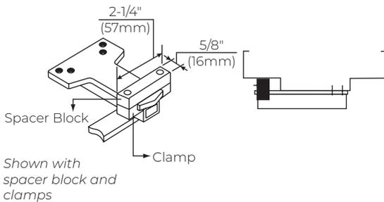
**Wide Frame - 6191 Reinforcing Kit:** Optional for use with all Unitrol parallel arms. Used to support the soffit plate on installations with deep frames. Clamps may be used with or without the spacer block, depending on frame conditions.
