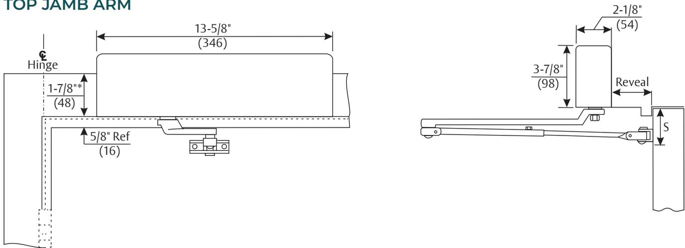
Mounting holes for closer body are spaced 2-3/8" (86mm) vertically x 6-3/4" (171mm) horizontally.
