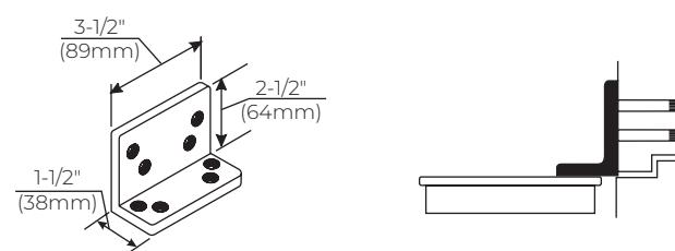
**Flush Rabbeted Transom - 2022 Angle Bracket:** Optional for use with all Unitrol parallel arms. For use where rabbeted or flush transom conditions prevent installation of the soffit plate assembly. This bracket fastens to the overhead transom to provide a mounting surface for the soffit plate assembly.
