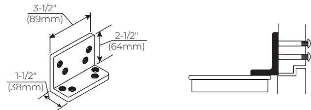
**Flush Rabbeted Transom - 2022 Angle Bracket:** Optional for use with all Unitrol parallel arms. For use where rabbeted or flush transom conditions prevent installation of the soffit plate assembly. This bracket fastens to the overhead transom to provide a mounting surface for the soffit plate assembly.
