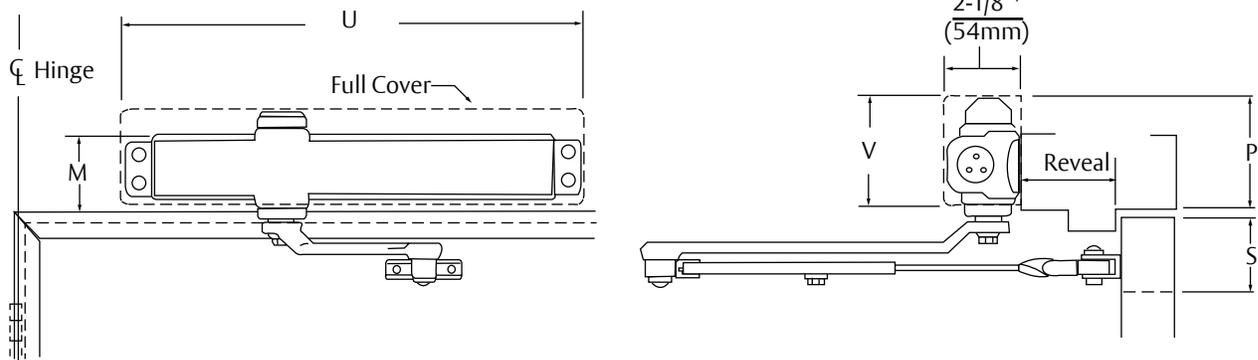
Mounting holes for closer body are spaced 3/4" (19mm) vertically x 12" (305mm) horizontally.
