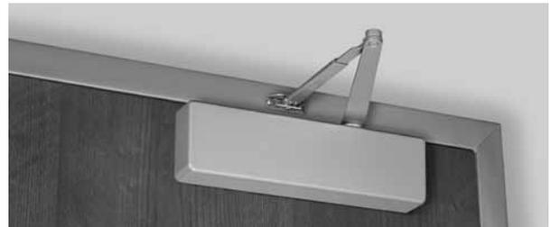
Regular Arm - allows closer to be installed where there is as little as 1" (25mm) of frame face or ceiling clearance.
