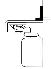
**Parallel Hold Open - 1628H Adapter Plate:** Supplied standard with all parallel arm hold open closers. It can also be used to convert regular arm or top jamb hold open arms to parallel arm installation. It can be mounted where the frame soffit is as narrow as 1" (25mm).
