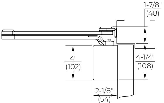
Mounting holes for closer body are spaced 2-3/8" (60mm) vertically x 6-3/4" (171mm) horizontally.
