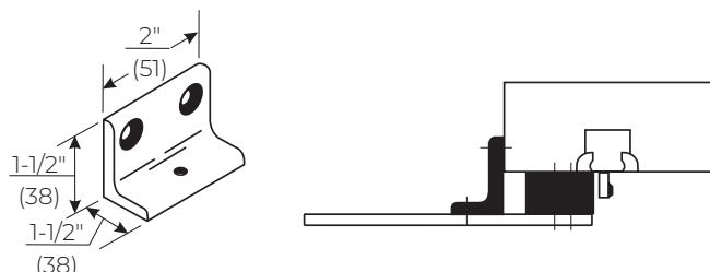
**Narrow Frame - 6890 Support Bracket:** For use where the frame is narrow, and the soffit plate cannot be mounted directly to the frame soffit or rabbet. Used in combination with the 6891 Spacer Block on blade stop frames to provide extra support and needed clearance of the blade stop.
