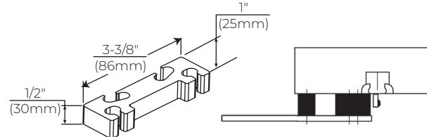
**Clearance/Support Blade Stop - 6891 Spacer Block:** For use where the door frame has a blade stop and the soffit plate must be mounted on the frame rabbet. This accessory is used in combination with the standard 2019S Spacer Block to provide clearance of the blade stop. For clearance of 5/8" (16mm) high-frame stop.
