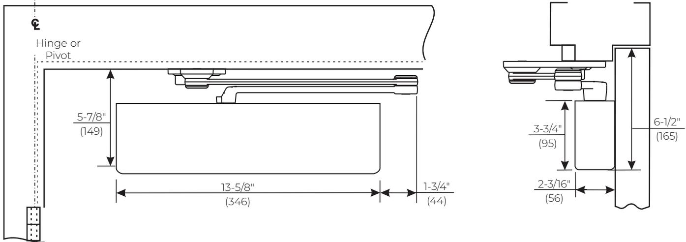
Mounting holes for closer body are spaced 2-3/8" (60mm) vertically x 6-3/4" (171mm) horizontally.
