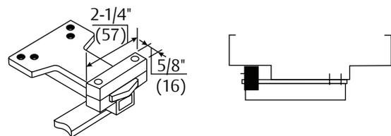
**Wide Frame - 6191 Reinforcing Kit:** Optional for use with all Unitrol parallel arms. Used to support the soffit plate on installations with wide frames. Clamps may be used with or without the spacer block, depending on frame conditions.
