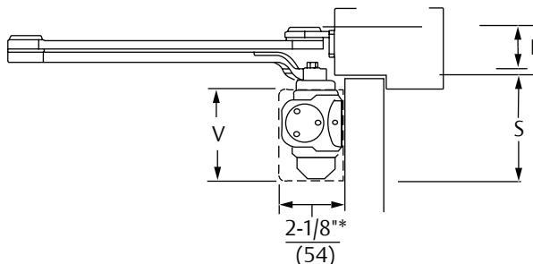
Mounting holes for closer body are spaced 3/4" (19mm) vertically x 12" (305mm) horizontally.
