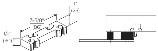
**Clearance/Support Blade Stop - 6891 Spacer Block:** For use where the door frame has a blade stop and the soffit plate must be mounted on the frame rabbet. This accessory is used in combination with the standard spacer block to provide clearance of the blade stop.
