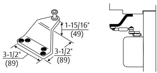
**Flush Transom - 2022 Angle Bracket:** For use where rabbeted or flush transom conditions prevent installation of a soffit plate. Used in combination with the 1618 soffit plate, or may be used in combination with the 2018S soffit plate when it is necessary for the closer arm to clear a separate overhead door holder.
