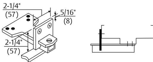
**Additional Support - 6190 Reinforcing Bracket:** Standard for use with all Unitrol parallel arms. Provides additional support to the soffit plate on installations with door frame reveals from 1-7/8" to 4-5/8" (48 to 117mm).
