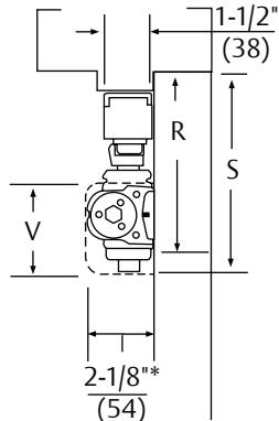
Mounting holes for closer body are spaced 3/4" (19mm) vertically x 12" (305mm) horizontally.
