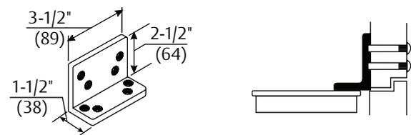
**Flush Rabbeted Transom - 2022 Angle Bracket:** Optional for use with all Unitrol parallel arms. For use where rabbeted or flush transom conditions prevent installation of the soffit plate assembly. This bracket fastens to the overhead transom to provide a mounting surface for the soffit plate assembly.
