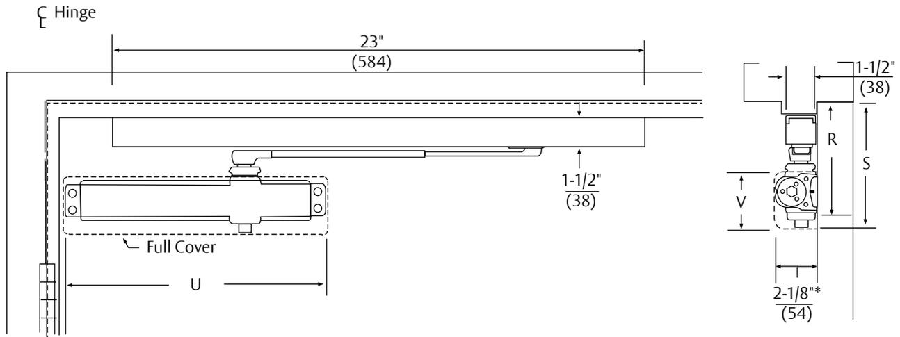
Mounting holes for closer body are spaced 3/4" (19mm) vertically x 12" (305mm) horizontally.
