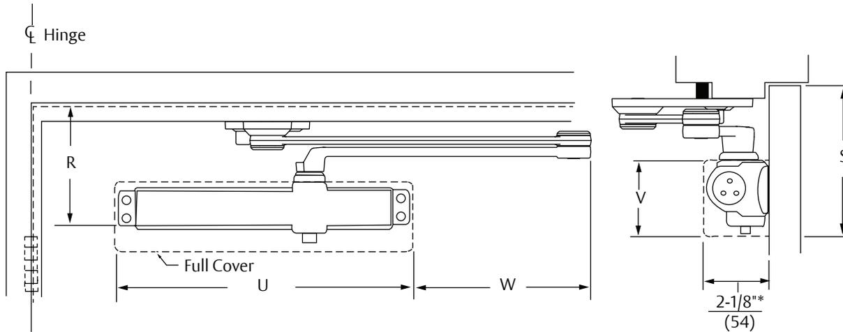
Mounting holes for closer body are spaced 3/4" (19mm) vertically x 12" (305mm) horizontally.
