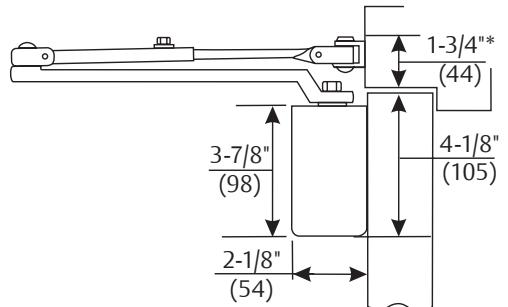
Mounting holes for closer body are spaced 2-3/8" (60mm) vertically x 6-3/4" (171mm) horizontally.
