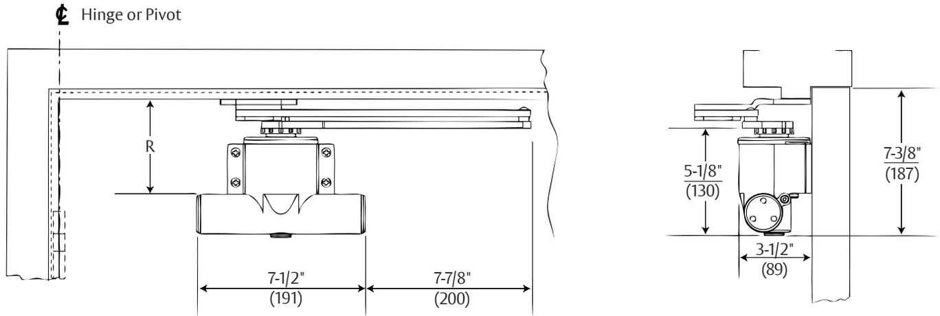
Body mounting holes are spaced 4-1/8" (105mm) horizontally and 1-3/8" (76mm) vertically.
