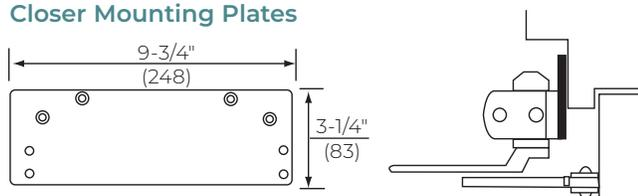
**Overhead Door Holder - 1688 Drop Plate:** For use where an overhead door holder prevents normal top jamb mounting. This places the center line of the arm mounting screws at 3-1/2" (89mm) from the top of the door.
