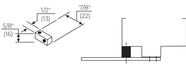
**Standard - 2019S Spacer Block:** For use where a narrow frame soffit does not provide adequate support for the soffit plate. Supplied as standard with all Parallel Rigid arm closers.
