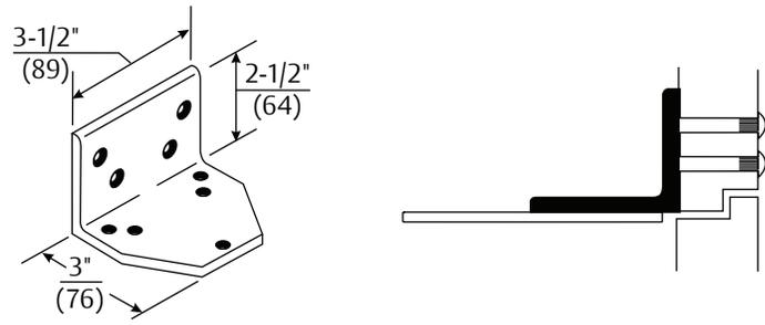
**Standard - 2019S Spacer Block:** For use where a narrow frame soffit does not provide adequate support for the soffit plate. Supplied as standard with all Parallel Rigid arm closers.
