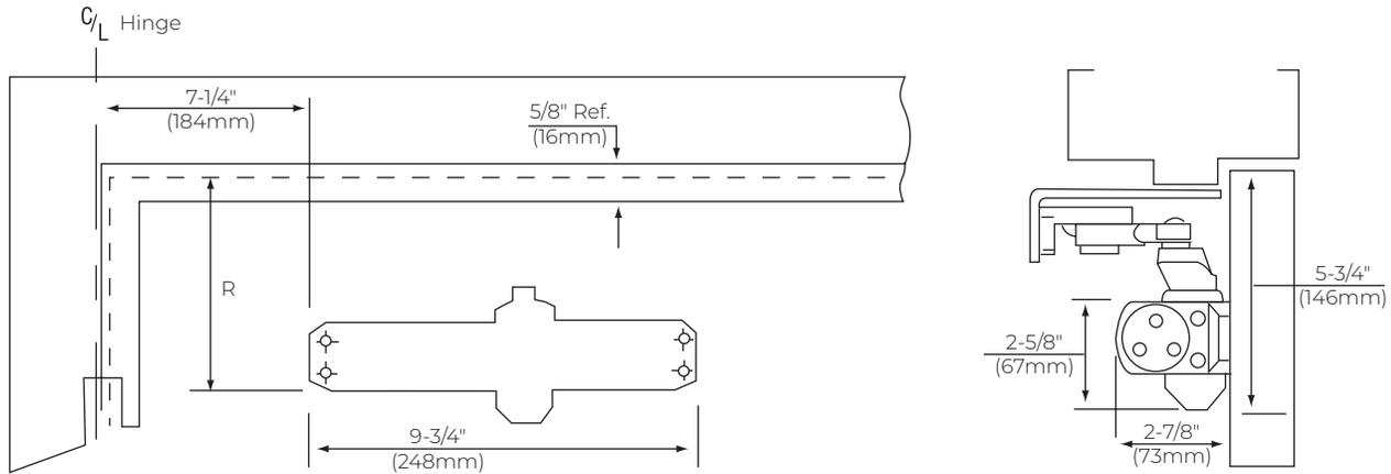
Mounting holes for closer body are spaced  $\frac{3}{4}$ " (19mm) vertically x  $9\text{-}\frac{1}{16}$ " (230mm) horizontally.
