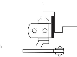
**Overhead Door Holder - 1688 Drop Plate:** For use where a overhead door holder prevents normal top jamb mounting. This places the center line of the arm mounting screws at 3-1/2" (89mm) from the top of the door.
