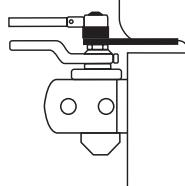
**Molded/Bull Nose Trim - 2403B Bracket:** For use where the door frame has molded or bull nose trim which will not accept a standard non-hold open shoe. The bracket is mortised into the frame rabbet, and projects beyond the face of the frame. It will accommodate a frame rabbet up to 2" (51mm) deep.
