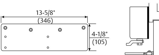
**Minimum Ceiling Clearance - 7787 Drop Plate:** For use where the ceiling clearance is as little as 1-7/8" (48mm).
