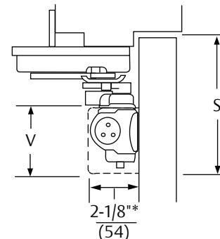
Mounting holes for closer body are spaced 3/4" (19mm) vertically x 12" (305mm) horizontally.
