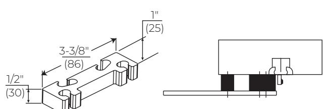
**Narrow Frame - 6890 Support Bracket:** For use where the frame is narrow, and the soffit plate cannot be mounted directly to the frame soffit or rabbet. Used in combination with the 6891 Spacer Block on blade stop frames to provide extra support and needed clearance of the blade stop.
