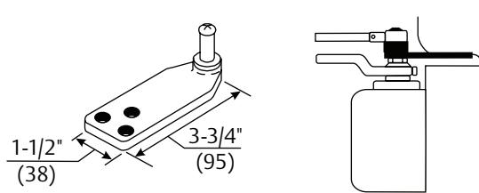
**Molded/Bull Nose Trim - 2403B Bracket:** For use where the door frame has molded or bull nose trim which will not accept a standard non-hold open shoe. The bracket is mortised into the frame rabbet, and projects beyond the face of the frame. It will accommodate a frame rabbet up to 2" (51mm) deep.
