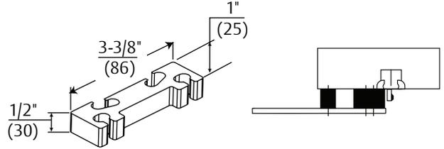
**Clearance/Support Blade Stop - 6891 Spacer Block:**
