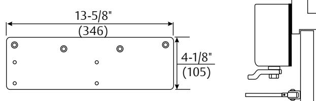
**Narrow Frame - 7786 Back Plate:** For use where a narrow frame face prevents the closer from being mounted directly to the frame. This back plate must be used for closer mounted on a frame between 1-7/8" and 3-1/8" (48 and 79mm) in height.
