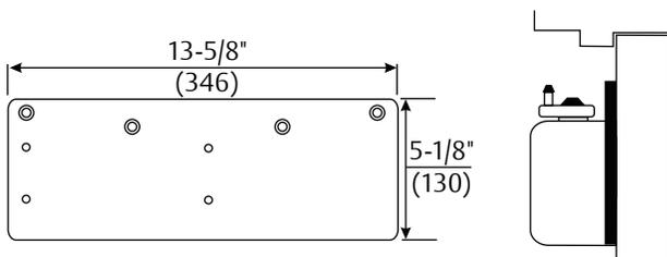
**Narrow Top Rail - 7788 Drop Plate:** For use where a narrow top rail prevents the closer from being mounted directly to the door surface. This drop plate can be used to mount a closer on a top rail as narrow as 2-3/8" (60mm) in height.
