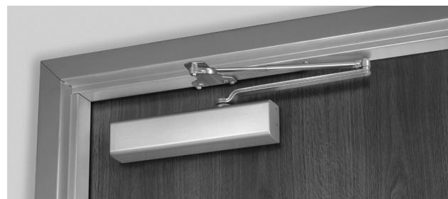
Due to the geometry of the arm it is approximately 25% less power efficient than a regular arm application. The entire closer and arm assembly are mounted below the frame stop. Top rail clearance dimensions will vary based on the type of cover used.
