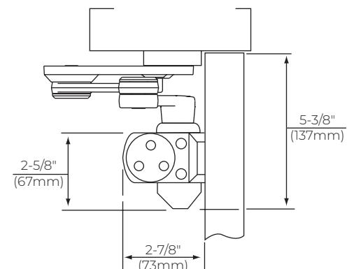
Mounting holes for closer body are spaced 3/4" (19mm) vertically x 9-1/16" (230mm) horizontally.
