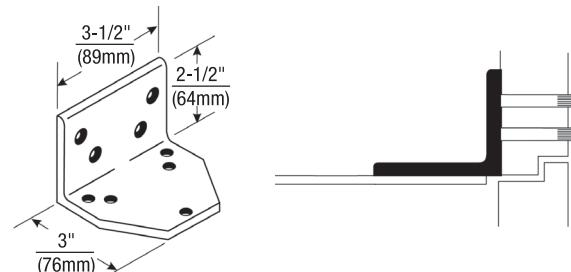
**Standard - 2019S Spacer Block:** For use where a narrow frame soffit does not provide adequate support for the soffit plate. Supplied as standard with all Parallel Rigid arm closers. For use on frame with either 1/2" (13mm) or 5/8" (16mm) high frame stop.
