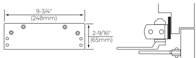
**Low Ceiling Clearance - Overhead Door Holder - 1687 Drop Plate:** For use where the ceiling clearance is between 1-3/4" and 2-5/8" (44 and 67mm). Or for use where an overhead door holder prevents normal top jamb mounting. This places the centerline of the arm mounting screws at 2-1/8" (54mm) from the top of door.
