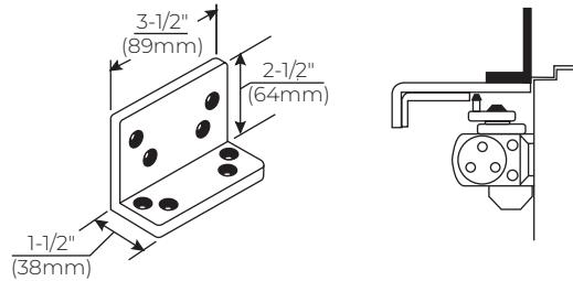
**Parallel Hold Open - 1628H Adapter Plate:** This Adapter Plate is supplied standard with all parallel arm hold open closers. It can also be used to convert regular arm or top jamb hold open arms to parallel arm installation. It can be mounted where the frame soffit is as narrow as 1" (25mm).
