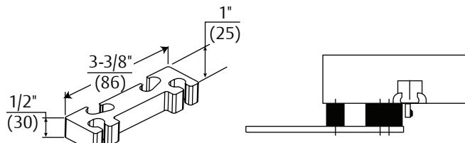
**Clearance/Support Blade Stop - 6891 Spacer Block:** For use where the door frame has a blade stop and the soffit plate must be mounted on the frame rabbet. This accessory is used in combination with the standard spacer block to provide clearance of the blade stop.
