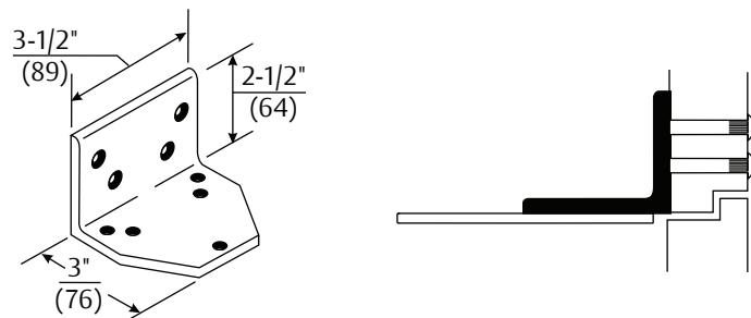
**Flush Rabbeted Transom - 2019L Angle Bracket:** For use where flush transom conditions prevent mounting of the standard soffit plate. This bracket is used in combination with the standard soffit plate.
