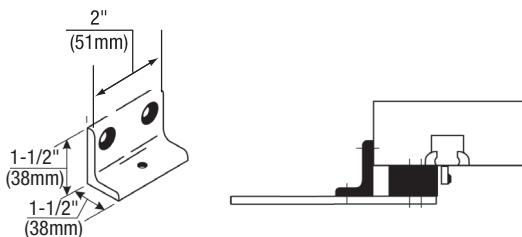
**Narrow Frame - 6890 Support Bracket:** For use where the frame is narrow and the soffit plate cannot be mounted directly to the frame soffit or rabbet. Used in combination with the 6891 Spacer Block on blade stop frames to provide extra support and needed clearance of the blade stop. Used on frame where frame stop does not exceed 5/8" (16mm) in height.
