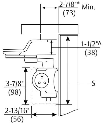
Mounting holes for closer body are spaced 2-3/8" (60mm) vertically x 6-3/4" (171mm) horizontally.
