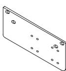
**410PDP** Narrow Top Rail Drop Plate (parallel arm): Required for parallel arm mounting where top rail is less than 5-1/2" (140mm), measured from the stop. Plate requires 2" (51mm) minimum top rail.
