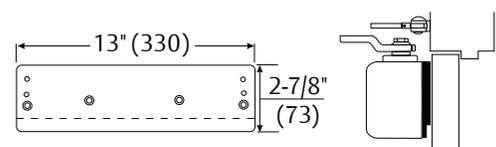
**Exposed Back/Narrow Top Rail - Exposed Back Concealed Door Holder - 8446 Molded Full Cover Drop Plate Kit:**
