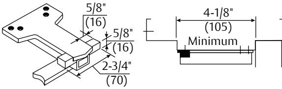
**Wide Frame - 6191 Reinforcing Kit:** Optional for use with all Unitrol parallel arms. Used to support the soffit plate on installations with wide frames. Clamps may be used with or without the spacer block, depending on frame conditions.
