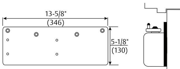
**Narrow Top Rail - 7788 Drop Plate:** For use where a narrow top rail prevents the closer from being mounted directly to the door surface. This drop plate can be used to mount a closer on a top rail as narrow as 2-1/2" (64mm) in height.
