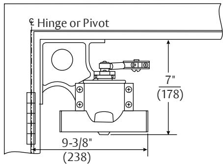
**Corner Mounting, Standard Drop - 2-B/F Corner Bracket:**
