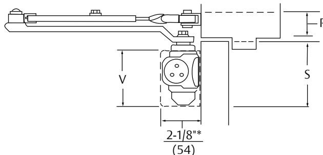
Mounting holes for closer body are spaced 3/4" (19mm) vertically x 12" (305mm) horizontally.
