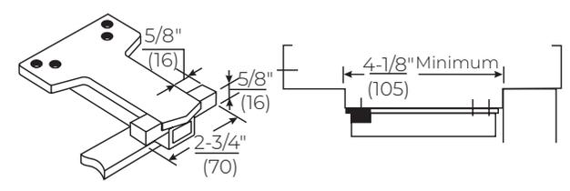
**Wide Frame - 6191 Reinforcing Kit:** Optional for use with all Unitrol parallel arms. Used to support the soffit plate on installations with wide frames. Clamps may be used with or without the spacer block, depending on frame conditions.
