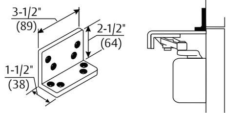
**Parallel Hold Open - 1628H Adapter Plate:** Supplied standard with all parallel arm hold open closers. It can also be used to convert regular arm or top jamb hold open arms to parallel arm installation. It can be mounted where the frame soffit is as narrow as 1" (25mm).
