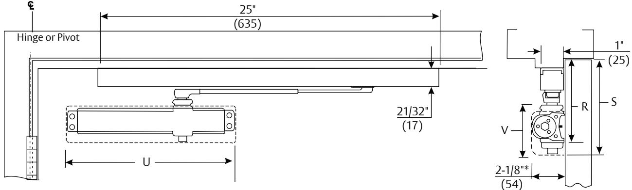
Mounting holes for closer body are spaced 3/4" (19mm) vertically x12" (305mm) horizontally.
