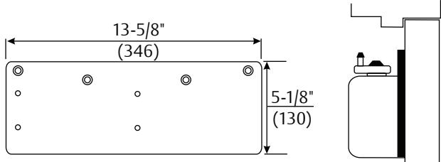
**Narrow Top Rail - 7788 Drop Plate:** For use where a narrow top rail prevents the closer from being mounted directly to the door surface. This drop plate can be used to mount a closer on a top rail as narrow as 2-1/2" (64mm) in height.
