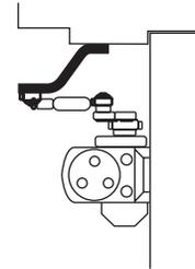
**Flush Transom - 2022 Angle Bracket:** For use where rabbeted or flush transom conditions prevent installation of a soffit plate. Used in combination with the 1618A soffit plate, or may be used in combination with the 2018S soffit plate when it is necessary for the closer arm to clear a separate overhead door holder.
