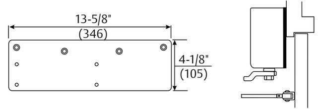
**Low Ceiling Clearance - Overhead Door Holder - 7787 Drop Plate:** For use where the ceiling clearance is between 1-7/8" and 3-7/8" (48 and 98mm) or where a surface or concealed overhead door holder prevents normal top jamb mounting. This plate drops the closer and allows the arm mounting screws to clear the bottom of the door holder. This places the centerline of the arm mounting screws at 3-1/8" (79mm) from the top of the door.
