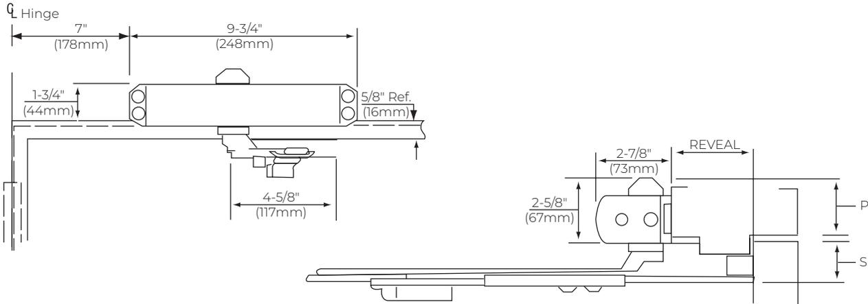
Mounting holes for closer body are spaced 3/4" (19mm) vertically x 9-1/16" (230mm) horizontally.
