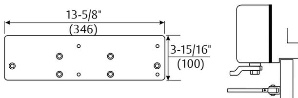
**Standard Installation - 7786 Back Plate:** Can be mounted where a frame face is as narrow as 1-5/8" (41mm) in height.
