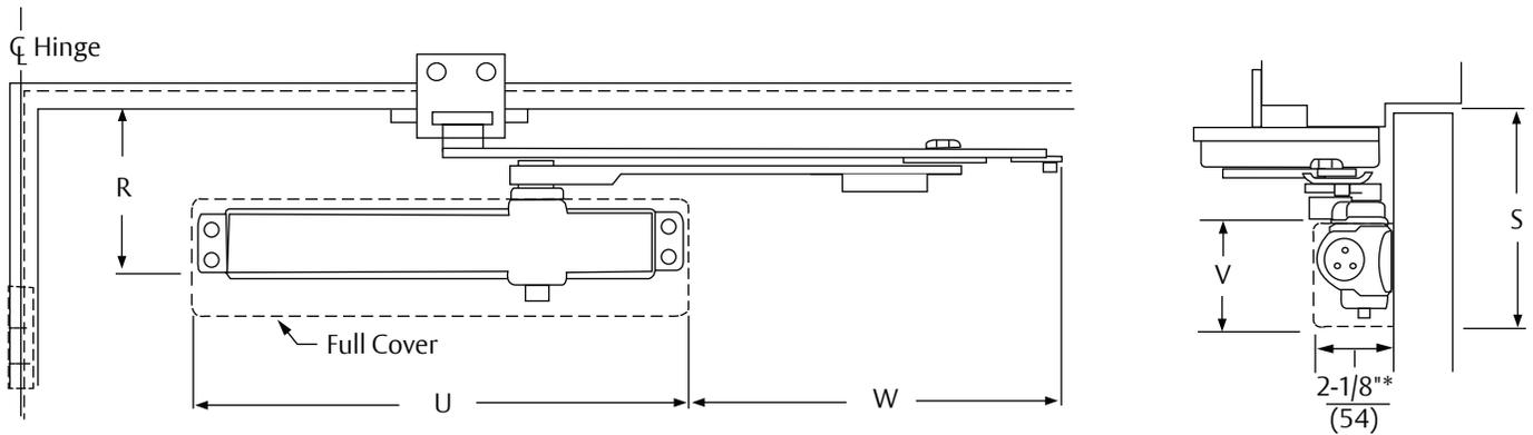
Mounting holes for closer body are spaced  $\frac{3}{4}$ " (19mm) vertically x 12" (305mm) horizontally.
