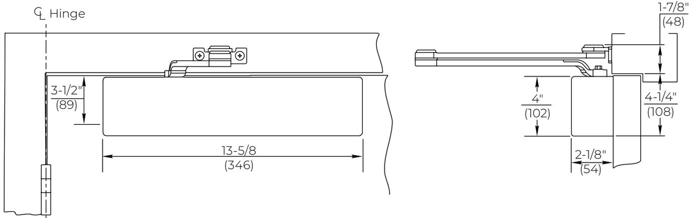
Mounting holes for closer body are spaced 2-3/8" (60mm) vertically x 6-3/4" (171mm) horizontally.
