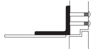
**Standard - 2019S Spacer Block:** For use where a narrow frame soffit does not provide adequate support for the soffit plate. Supplied standard with all Parallel Rigid arm closers.
