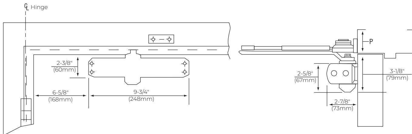
Mounting holes for closer body are spaced 3/4" (19mm) vertically x 9-1/16" (230mm) horizontally.
