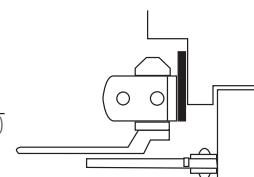
**Low Ceiling Clearance - 1687 Drop Plate:** For use where the ceiling clearance is between 1-3/4" and 2-5/8" (44 and 67mm). This places the centerline of the arm mounting screws at 2-5/8" (67mm) from the top of door.
