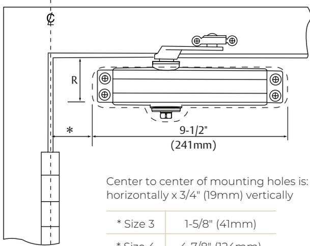
Center to center of mounting holes is: 8" (203mm) horizontally x 3/4" (19mm) vertically
