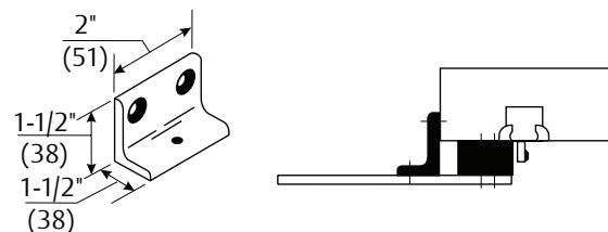
**Narrow Frame - 6890 Support Bracket:** For use where the frame is narrow, and the soffit plate cannot be mounted directly to the frame soffit or rabbet. Used in combination with the 6891 Spacer Block on blade stop frames to provide extra support and needed clearance of the blade stop. Used on frames where the frame stop does not exceed 5/8" (11mm) in height.
