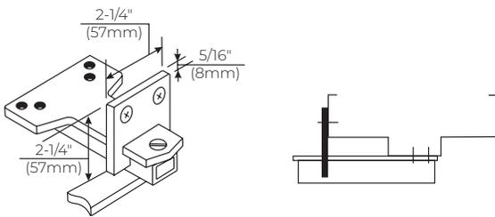
**Additional Support - 6190 Reinforcing Bracket:** Standard for use with all Unitrol parallel arms. Provides additional support to the soffit plate on installations with door frame reveals from 1-7/8" to 4-5/8" (48 to 117mm).
