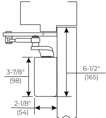
Mounting holes for closer body are spaced 2-3/8" (86mm) vertically x 6-3/4" (171mm) horizontally.
