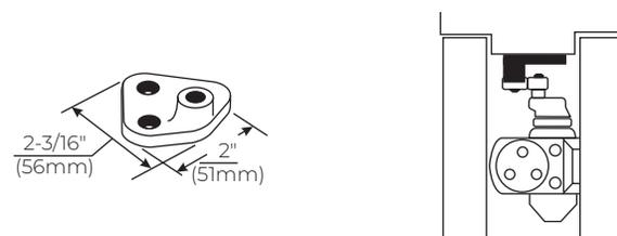
**Standard Installation - 1618A Soffit Plate:** This soffit plate is supplied standard with parallel arm closers. It can be mounted where the frame soffit is as narrow as 1" (25 mm).
