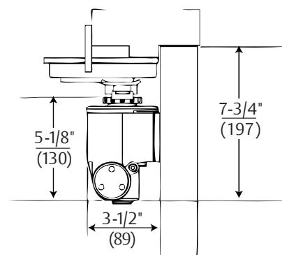
Body mounting holes are spaced 4-1/8" (105mm) horizontally and 1-3/8" (76mm) vertically.
