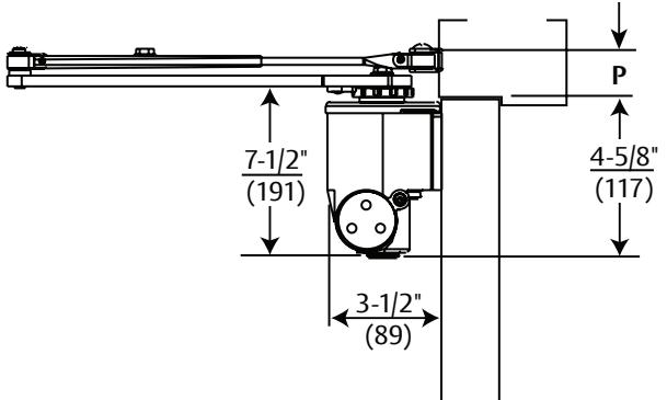
Body mounting holes are spaced 4-1/8" (105mm) horizontally and 1-3/8" (76mm) vertically.
