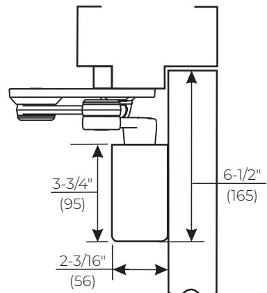
Mounting holes for closer body are spaced 2-3/8" (60mm) vertically x 6-3/4" (171mm) horizontally.
