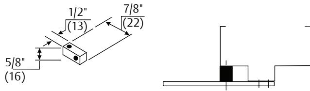
**Standard - 2019S Spacer Block:** For use where a narrow frame soffit does not provide adequate support for the soffit plate. Supplied as standard with all Parallel Rigid arm closers.
