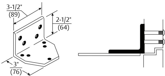
**Flush Rabbeted Transom - 2019L Angle Bracket:** For use where flush transom conditions prevent mounting of the standard soffit plate. This bracket is used in combination with the standard soffit plate.
