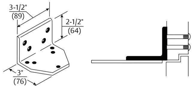
**Standard - 2019S Spacer Block:** For use where a narrow frame soffit does not provide adequate support for the soffit plate. Supplied as standard with all Parallel Rigid arm closers.
