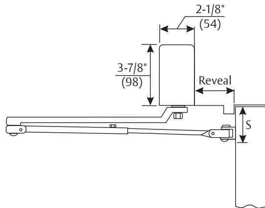
Mounting holes for closer body are spaced 2-3/8" (86mm) vertically x 6-3/4" (171mm) horizontally.
