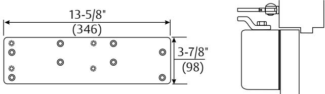
**Narrow Top Rail - 7786 Drop Plate:** For use where the narrow top rail of the door prevents the closer from being mounted directly to the door surface. This drop plate must be used for closer mounted on a top rail between 1-7/8" and 3-3/8" (48 and 86mm) in height.
