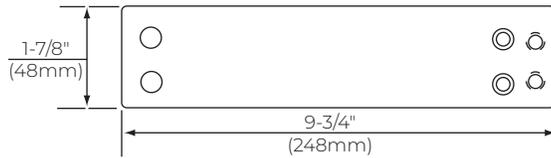
**1699 Adapter Plate:** Converts old 1602/1603 closer installations with 3/4" (19mm) x 8-3/16" (208mm) - spacing to new 1603 using existing mounting holes in door or frame.
