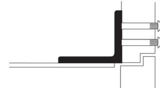
**Flush Rabbeted Transom - 2019L Angle Bracket:** For use where flush transom conditions prevent mounting of the standard soffit plate. This bracket is used in combination with the arm's soffit plate.
