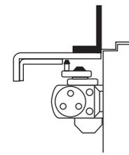
**Parallel Hold Open - 1628H Adapter Plate:** This Adapter Plate is supplied standard with all parallel arm hold open closers. It can also be used to convert regular arm or top jamb hold open arms to parallel arm installation. It can be mounted where the frame soffit is as narrow as 1" (25mm).
