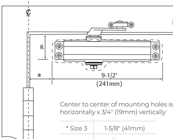
Center to center of mounting holes is: 8" (203mm)
