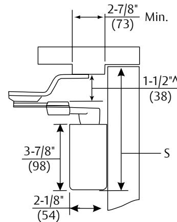
Mounting holes for closer body are spaced 2-3/8" (60mm) vertically x 6-3/4" (171mm) horizontally.
