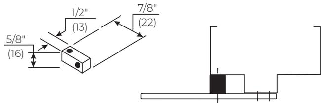
**Standard - 2019S Spacer Block:** For use where a narrow frame soffit does not provide adequate support for the soffit plate. Supplied as standard with all Parallel Rigid arm closers.
