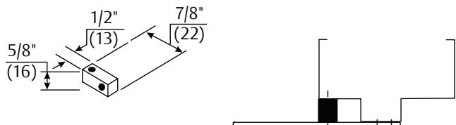
**Standard - 2019S Spacer Block:** For use where a narrow frame soffit does not provide adequate support for the soffit plate. Supplied as standard with all Parallel Rigid arm closers.
