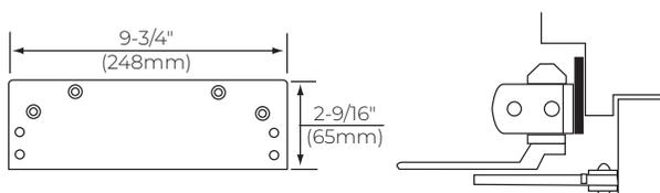
**Low Ceiling Clearance - 1687 Drop Plate:** For use where the ceiling clearance is between 1-3/4" and 2-5/8" (44 and 67mm). This places the centerline of the arm mounting screws at 2-5/8" (67mm) from the top of door.
