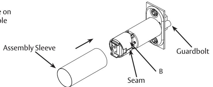
4. Test the deadlocking of the latch: Press and hold guardbolt. Latchbolt must block, if pressed. Test the retraction of the latch by pressing the guardbolt and pulling on tailpiece "F".
