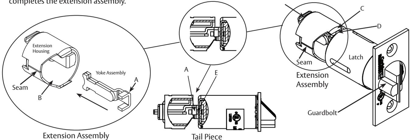
3. After assembly, the seam and cutaway "B" needs to be on the same side as deadlocking guardbolt. Then assemble sleeve to hold both latch and latch extension.
