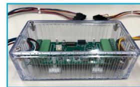
(SNT1) WTB OSDP adapter wiring harness
