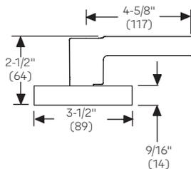
AU and PB levers comply with codes requiring lever to return to within 1/2" (13mm) of door face.
