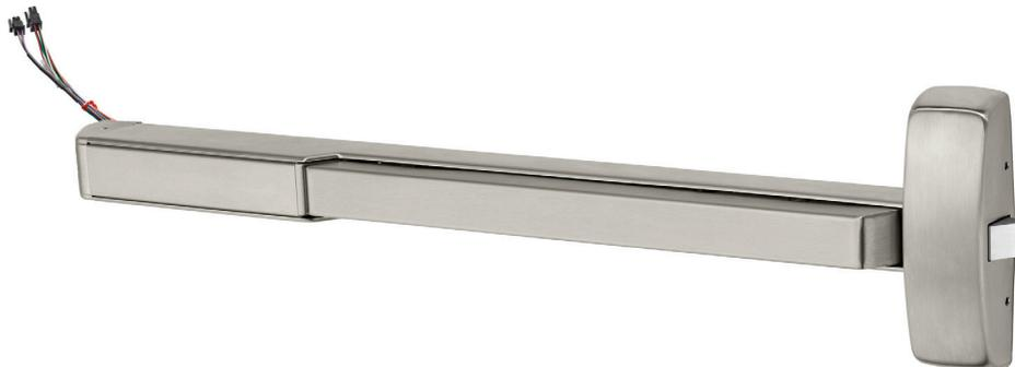
The Request-to-Exit option provides includes a signal switch to monitor if push rail is depressed. The switch can be used to activate a variety of features, such as sound and alarm, initialize a delay egress system, or de-energize an electromagnetic lock.
