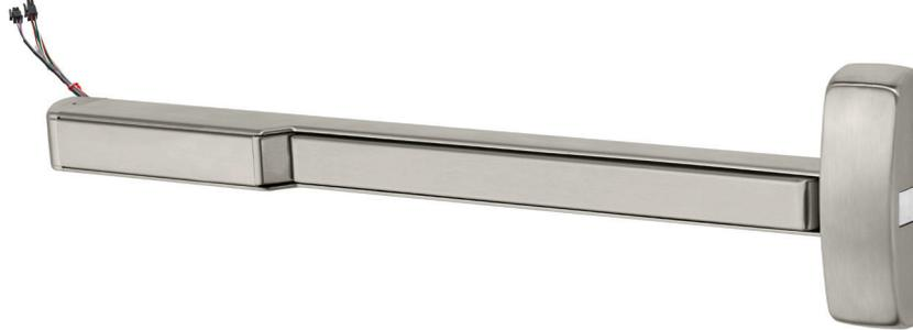
Libraries, auditoriums, theaters, courtrooms, churches and schools benefit from the convenience of electric dogging (unlocking). When the exit device is energized and the push rail is depressed, it will continuously hold the push rail down and the latch(es) will be held retracted. When the device is de-energized or power is interrupted, the latch(es) will extend. This feature is ideal for areas that require the silent operation of exit device hardware.
