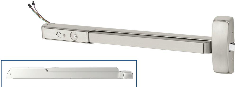
The 59- sounds an alarm within the rail when the exit device push pad is pressed down, in order to alert personnel that someone is attempting to exit. The exit device is preset to remain locked for 15 seconds, allowing time for authorized personnel to respond. This can be done by inserting a key into the cylinder on the rail or via a remote location. When the connected fire alarm system is activated, the exit device disarms and allows immediate egress.
