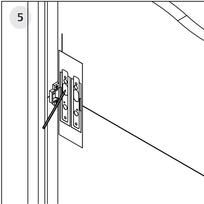
Place supplied paper template against the strike. Mark hole and mounting holes per device function.
