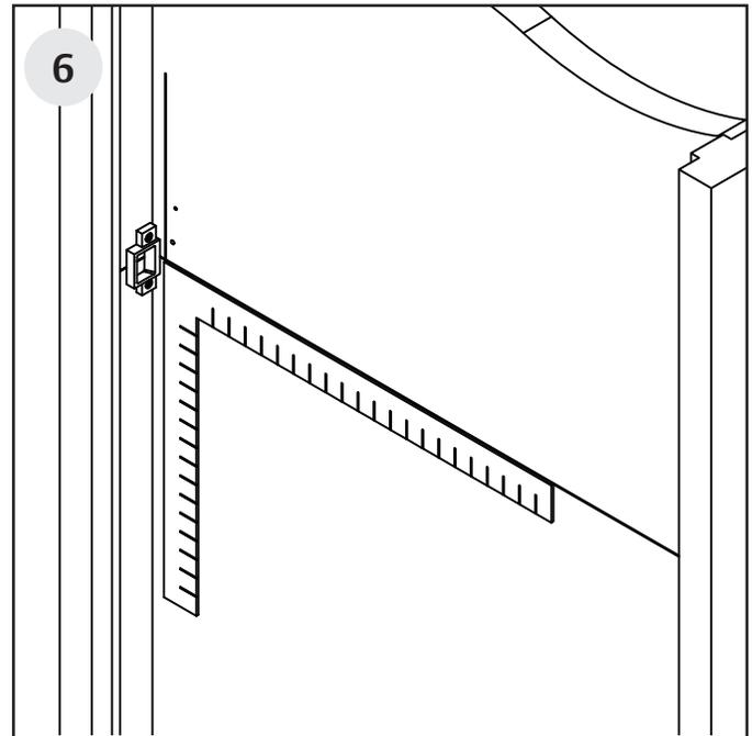
Using a square, extend centerline marks created in Step 1.
