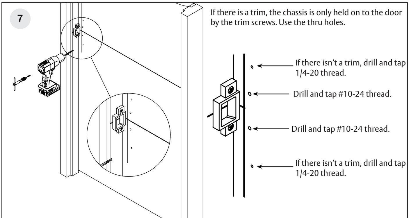
If there is a trim, the chassis is only held on to the door by the trim screws. Use the thru holes.
