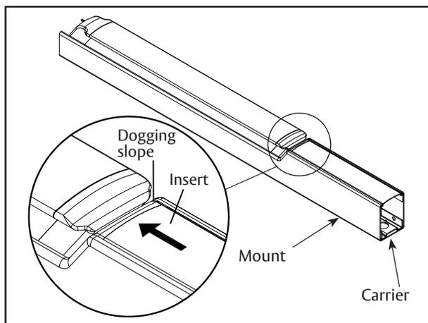
A. Ensure there isn't a gap between the insert and the dogging slope, and the carrier is flush with the mount.
