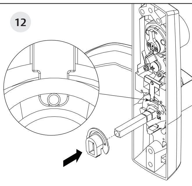
Insert the spindle lock. Make sure that the locking mechanism inserts into the slot.
