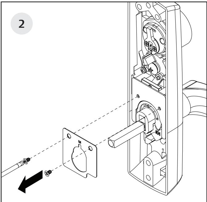
Loosen #4-40 x 3/16" flat head screws with a screwdriver. Remove the flat head screws and cover plate.
