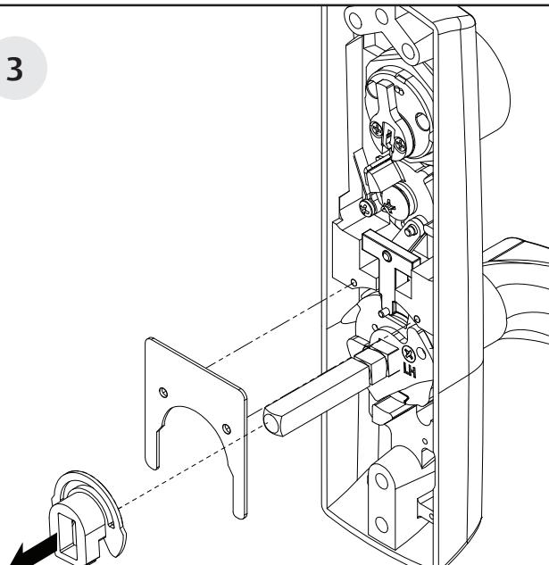
Remove the spindle lock and retaining plate.
