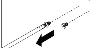
Remove two #4-40 x 3/16" flat head screws from the hub plate.
