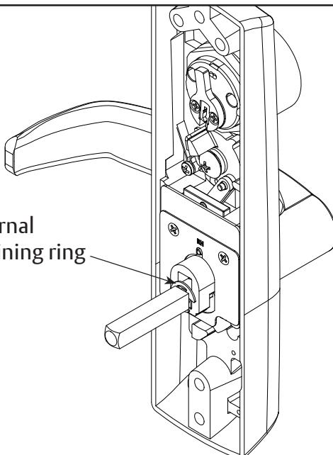
Reinstall the external retaining ring.
