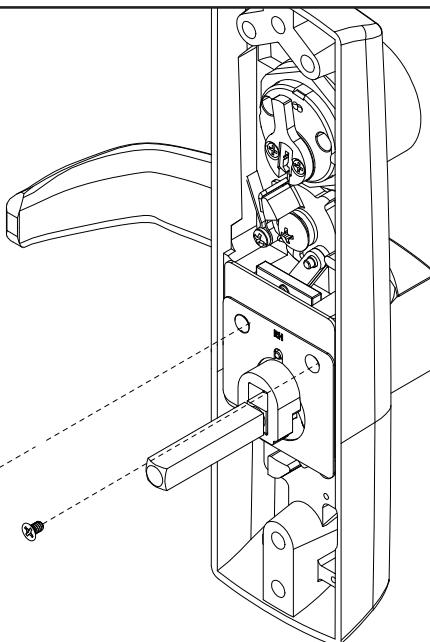
Secure the cover plate with two #4-40 x 3/16" flat head screws.
