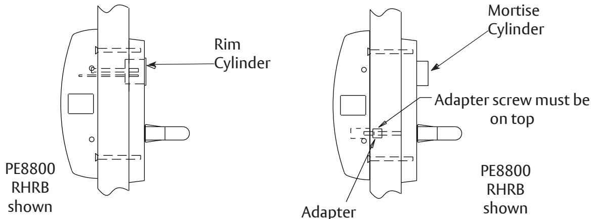
**Important:** See instruction sheet A8301 for (12-) PE8888 and (12-) HC-PE8800 and A8302 for PE8500 exit devices mounting. Securely fasten adapter to spindle with set screw before mounting.
