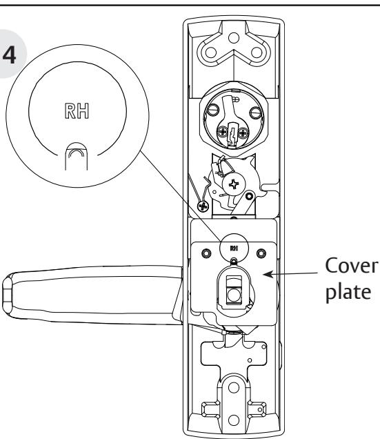
Determine the door handing, then reinstall the cover plate accordingly.
