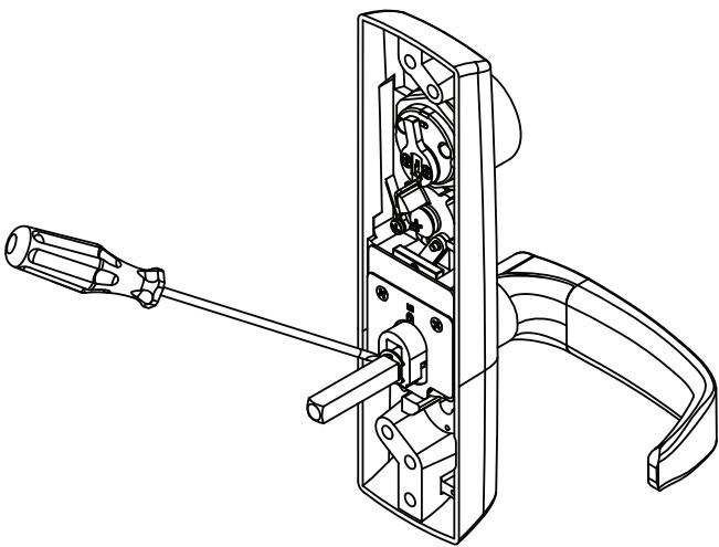
Remove the external retaining ring.
