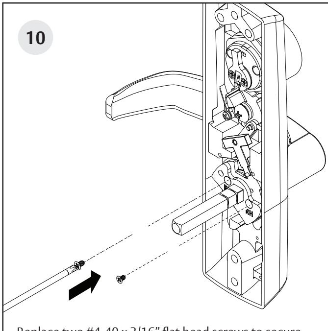
Replace two #4-40 x 3/16" flat head screws to secure the hub plate.
