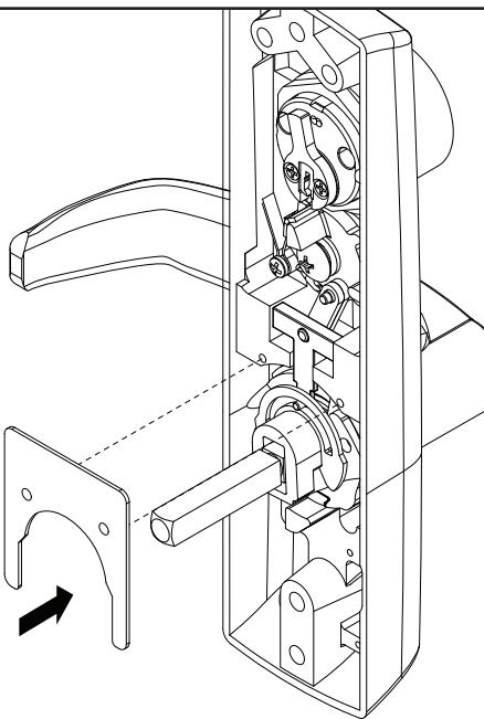
Reinstall the retainer plate.
