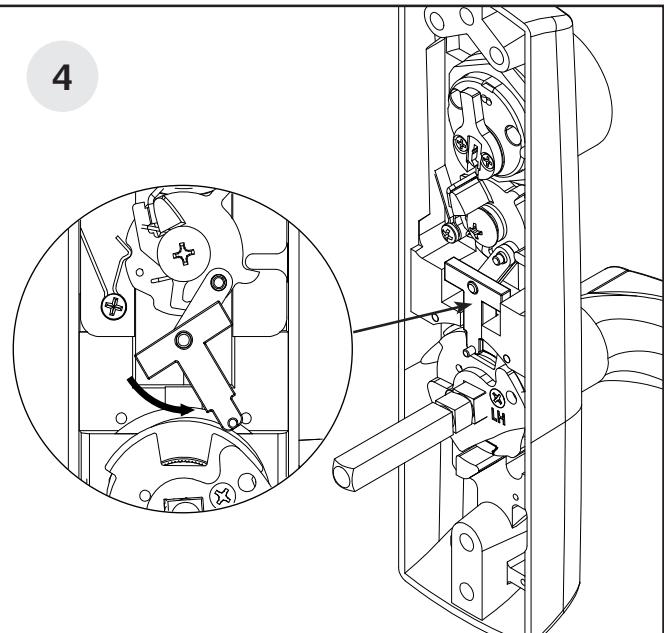
Push the locking mechanism to the right.
