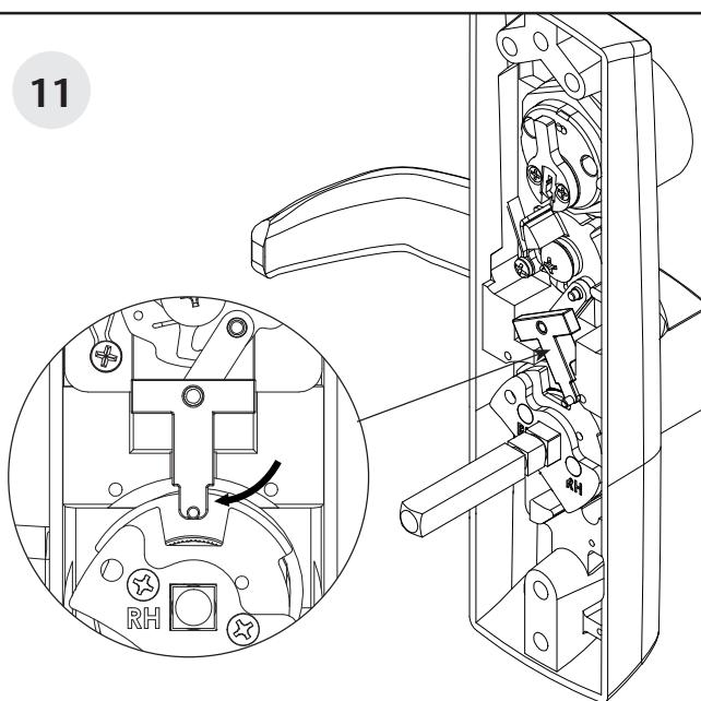
Move the locking mechanism to its original position.
