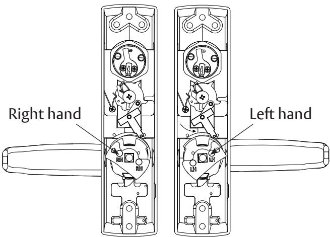
Turn the hub plate according to the door's handing.
