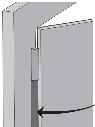
⚠ Complete protection of the side closing edge also invariably involves protection of the hinge side. We therefore recommend our hinge protection profiles, which are suitable for all hinge types.
