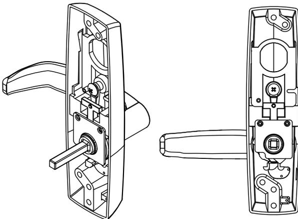
Insert bushing and then insert cover plate.
