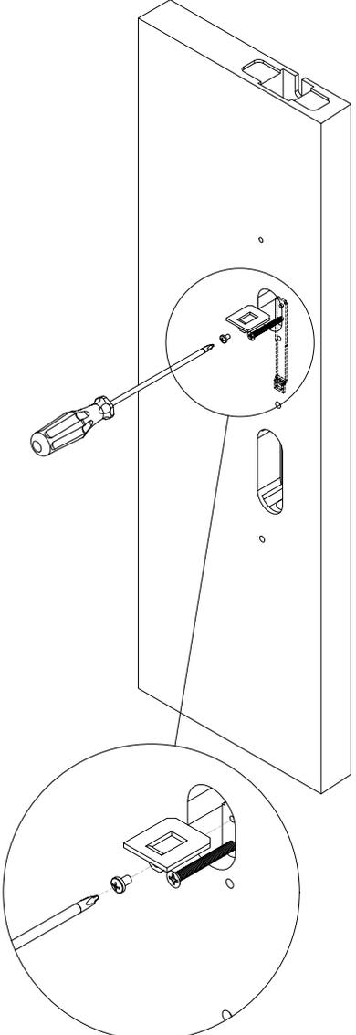
Holding the #10-32 fastener, take the platform and the smaller screw and attach it to the upper hole on the link in the door. Remove the #10-32 X 2" fastener.
