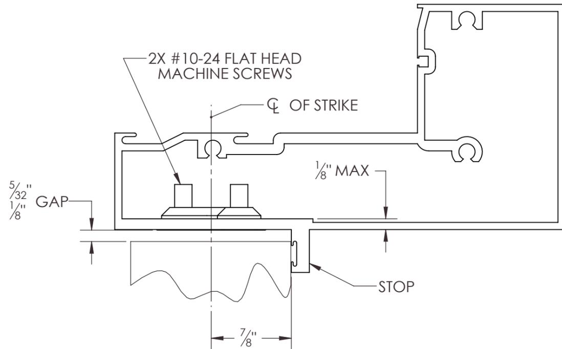
USE THIS DIMENSION WHEN DOOR STOPS AGAINST FRAME AS ILLUSTRATED. IF DOOR SILENCERS (RUBBER OR FELT BUMPERS) DOOR PANELS OR BOTH ARE USED, INCREASE THIS DIMENSION ACCORDINGLY.
