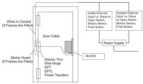
Operation: Activating inside or outside external input will retract latchbolt. Latchbolt remains retracted until power off.
