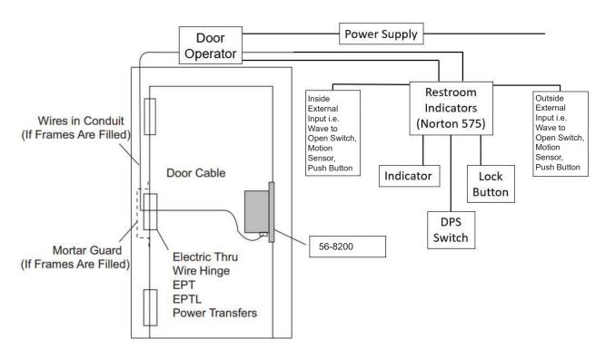
Operation: Activating inside or outside external input will retract latchbolt and door operator will open the door, unless outside external input is disabled by lock button. Indicator will illuminate when outside external input is disabled. Latchbolt remains retracted until power off.
