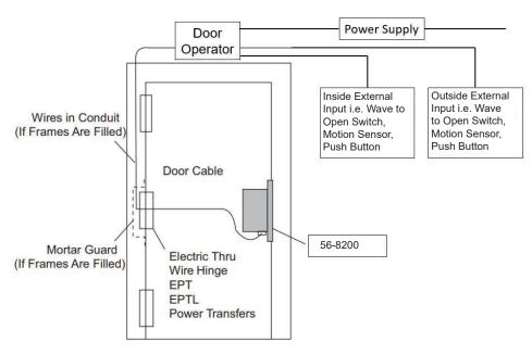
Operation: Activating inside or outside external input will retract latchbolt and door operator will open the door. Latchbolt remains retracted until power off.
