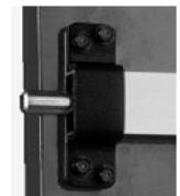
2 "Bullet" stationary bolts are provided for the locking points on the hinge-side of the door. As the door swings into the frame, the bolts project into the frame.
