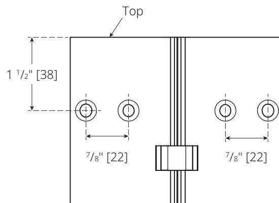
Additional clearance needed for bevelled edge hinge side of door.
