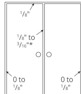
\*Allow extra clearance as required per astragal manufacturer. Certain door and frame conditions may require an extra  $\frac{1}{32}$ "- $\frac{1}{16}$ " clearance. Excessive clearance on fire rated assemblies may violate the requirements of NFPA 80.
