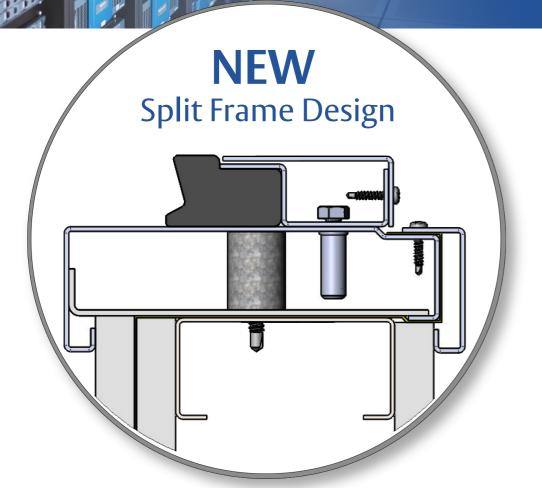
EMI-RFI/STC Shielding Assemblies with Split Frame and Adjustable Seals provide the best electromagnetic and radio-frequency protection for new and retrofit applications including SCIF compliance.
