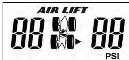
LCD with only right spring selected
