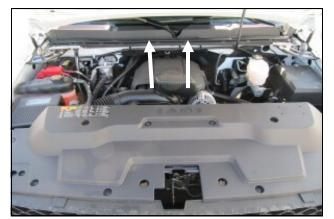
1. <u>Disconnect the negative battery cable.</u>
