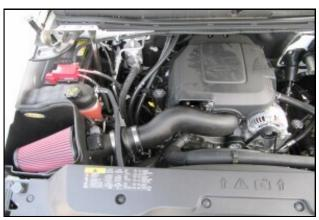
15. Reinstall the engine cover. Double check your work! Make sure there is no foreign material in the intake path. Make sure all clamps, hoses, bolts, and screws are tight. Double check the hood clearance. Reconnect the negative battery cable
