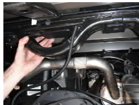
Figure 8.1: Axle Vent Hose Relocation
