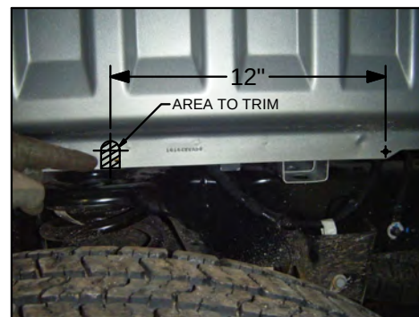
Figure 10.1: Inside Driver Side Rear Wheel Well
