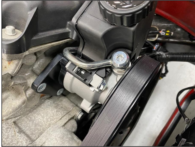
Figure 8 – Hardline Power Steering Pump Installed
