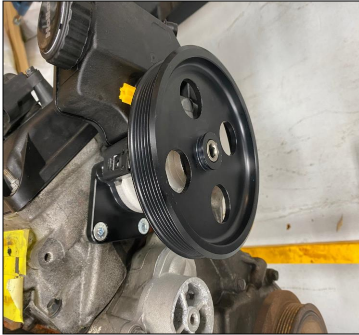
Figure 6 – 198-104/97-383 Assembly Installed onto 97-380 Adapter
