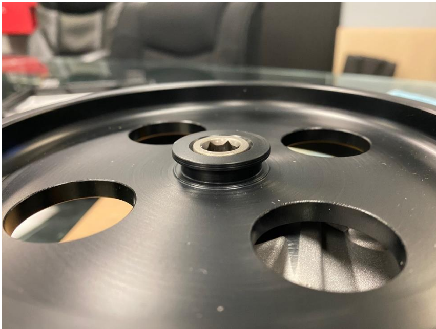
Figure 5 – 97-383 Pulley Installed onto 198-104 Power Steering Pump
