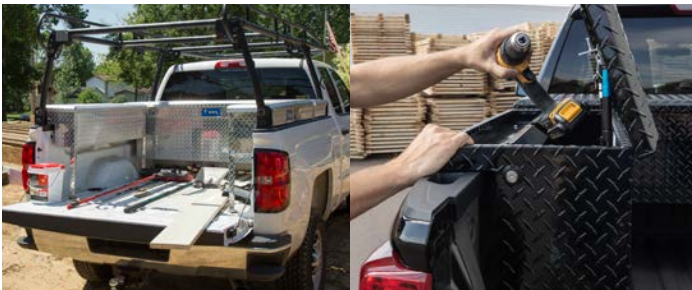
Truck side boxes provide a longer, shallower space for storage above the rear fender and are available with paddle handles (standard models only) or push-button operation (low-profile models only)
