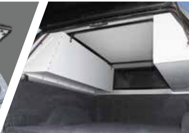
TOOLBOXES ARE SECURELY FASTENED TO ROOF FRAMEWORK
