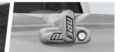
PALM HANDLE WITH SLAM LATCH SYSTEM
