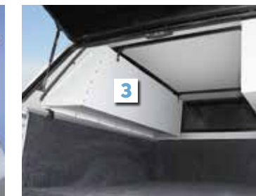
Toolboxes are securely fastened to roof framework
