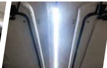
RIVAL LED ROPE LIGHT OPTION ACTIVATED WHEN ANY DOOR OPENS
