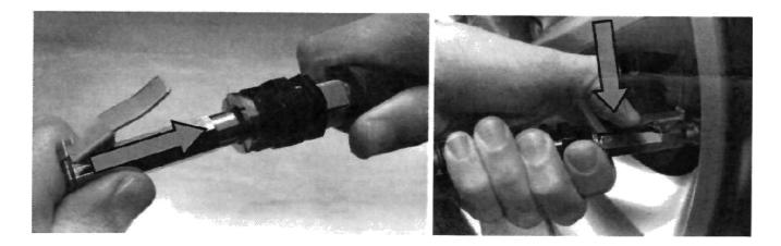
NOTE: Tire filler attachment is equipped with a stop valve, air will not pass through the tire filler attachment until it is connected to a tire valve.
