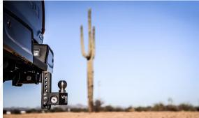
Steel Weigh Safe -6'' Drop Hitch with 2" Shank (8K/15K GTWR); Adjustable Ball Mount; Built-in Scale to Measure Tongue Weight; 15,000 lbs GTW
