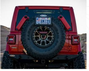
EZ RACK Kit, Basic — Steel; Mounts Any Tire, Carry Gas Kits, or Emergency Kits; Pre-Drilled Holes for Roto Pax/Daystar Storage Systems; RSE Jack and Shovel Mounts; Powder Coated Textured Black; 1/8 Steel; Made in the USA
