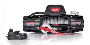
VR EVO 10-S Vehicle Recovery Winch — Vehicle Mounted; 12-Volt Electric; 10,000 Pound Line Pull Capacity; 90-Foot Synthetic Rope; Hawse Fairlead; Wired Remote; Planetary Gear Drive; Requires Winch Carrier or Winch Mount
