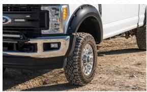
Pocket Style® Fender Flares — 4 pc.; Front Tire Coverage 1 in.; Front Height 5.5 in.; Rear Tire Coverage 1 in.; Rear Height 5.5 in.; Smooth Finish; Black
