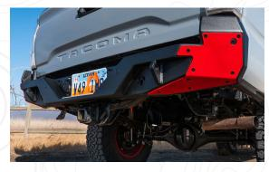
Toyota Tacoma 3G Rear Bumper – Powder-Coated; High-Clearance Rear Bumper For 3rd Gen Toyota Tacoma; Offers Tough Skid Plate Protection with Countersunk Hardware for a Smooth Surface; Comes in Bare Steel or Black Powder Coat
