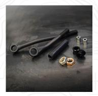
Available for Dodge and Ford Applications, Gas or Diesel; Eliminates "Death Wobble"; High-Quality Black Cerakote Finish to Resist Corrosion; Adjustable for Leveling and Lift Kits; Forged I-Beam Centerlink 30% Stronger than OEM, Tie Rods 1.5x Larger than OEM; Compatible with OEM Components
