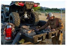
Drawer Storage System for Full Size Pickups; Two-Drawer Storage System; 75.25 in.; Made of High-Density Polyethylene; Stainless Steel Hardware; Features Cast Aluminum Handles/Galvanized Steel Subframe; Black XG7
