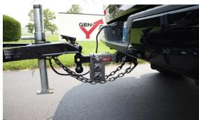
Mega-Duty 2" Shank 5" Offset Drop 2K TW 16K Hitch & GH-051 Dual-Ball & GH-032 — Adjustable; 10,000–32,000-lb. Towing Capacity; Multiple Drop Options
