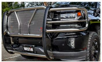
HDX Grille Guard Stainless Steel – 2 in. Diameter; Polished Stainless Steel
