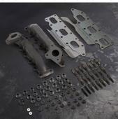
Eliminates Common Exhaust Leak by Utilizing All 11 Stud Locations; Improved Exhaust Flow; High-Silicon Ductile Iron Construction to Reduce Manifold Warping; Longer Fasters with Spacers that Reduce Stress During Heat Cycling and Prevent Bolts from Breaking; Machined Smooth Hardware Mating Surfaces to Further Prevent Hardware Failures; Kit Includes All Gaskets and Fasteners
