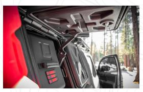
Second-generation, completely re-designed GearPOD has new features like a spring activated "Leitner Lid Lifter" for easy opening and closing, improved water-resistant seal, and re-engineered brackets for maximum strength. Installs easily on all Leitner Designs ACS racks using 4 TrakLOK nuts and grade 10.9 bolts.
