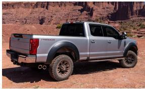
Extend-A-Fender® Style Fender Flares — 4pc; Front Tire Coverage 1.8 in.; Front Height 7.15 in.; Rear Tire Coverage 1.8 in; Rear Height 7.7 in.; Smooth Finish; Black
