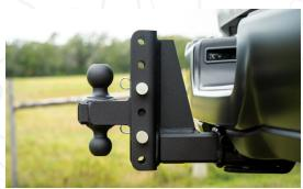
2.5" Heavy Duty, 6" Drop/Rise Class 5 Hitch with Pins and 2"/2-5/16"
