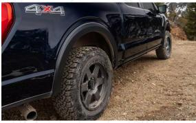
OE Style® Fender Flares — 4 pc.; Front Tire Coverage 0.75 in.; Front Height 3.5 in.; Rear Tire Coverage 0.75 in; Rear Height 4 in.; Smooth Finish; Black
