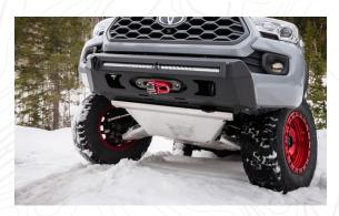
Toyota Tacoma 3G Bellypan Skid Plate — Built for Heavy-Duty Strength; Features Heat-Treated Aluminum Skid Plate & Steel Brackets
