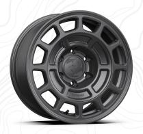
The Metrix HD — 12-Spoke, Open-Windowed Design; Deep Lug Bowl & Pocketed Valve Stem Seat; First fifteen52 Design with a Radial Reinforced Drop Center for Added Strength; Available in the Standard HD Specification with Fitments to Cover Most Popular 5- and 6-Lug Applications
