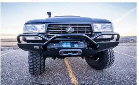
Hawse Fairlead 1.5 (1.5 Thick); Machined from 1.5-In Thick 6000 Series Aluminum; Large Outer Fillet Radius; Taller Rope Slot Height Opening
