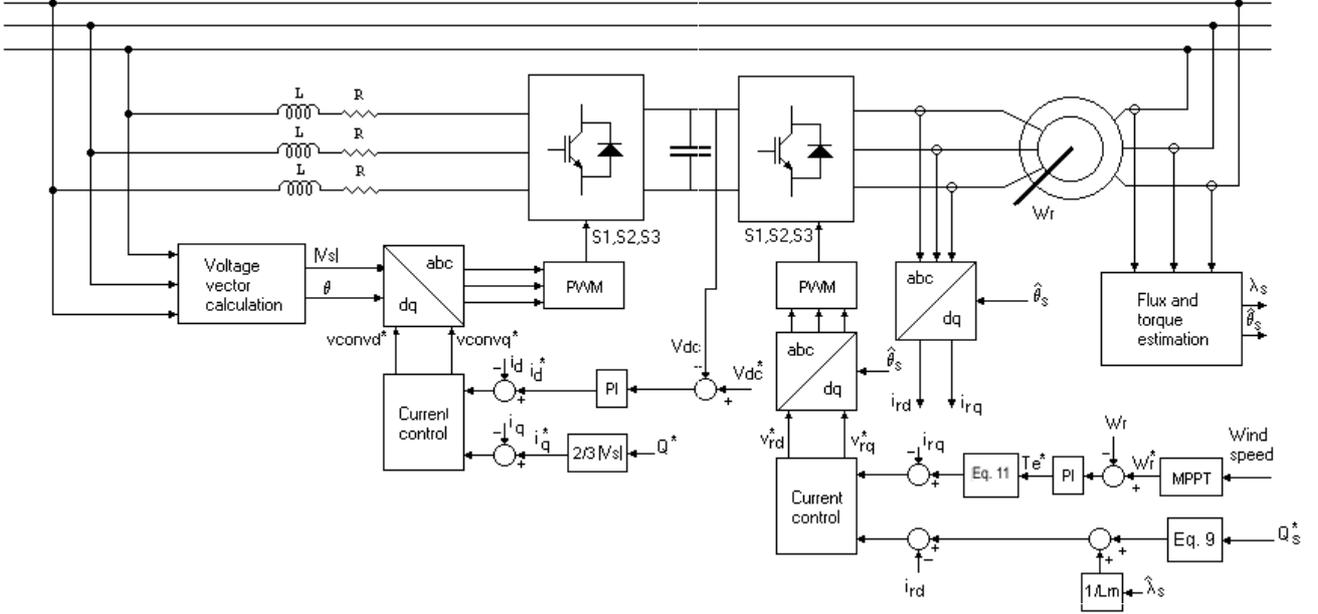
Fig. 1. Complete model of the generator and MSC and GSC control scheme.
