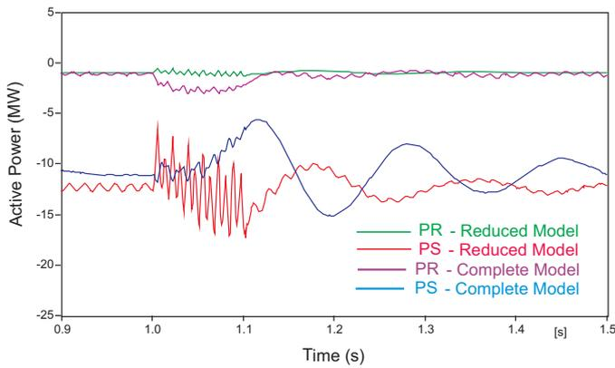
Fig. 8. Active power delivered to the stator terminals.
