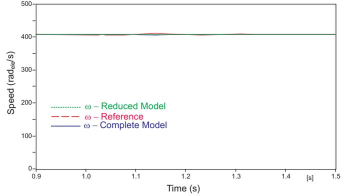
Fig. 6. Rotor electrical angular speed.
