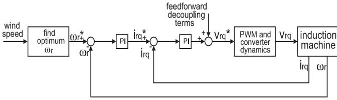
Fig. 5. Control scheme for MPPT in the complete model.
